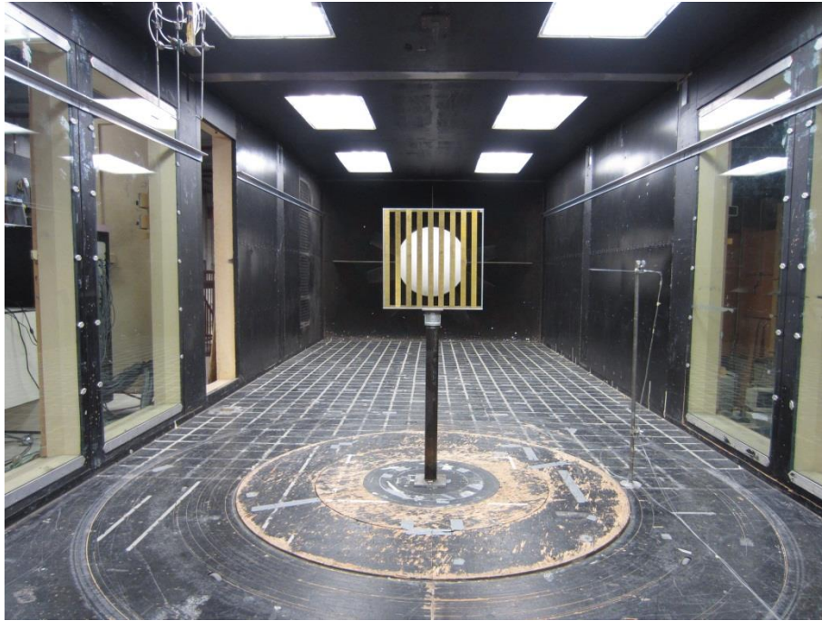
Figure 2.13. Photo of 2-D frame in the wind tunnel (configuration 30 shown).
