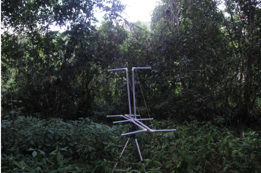
Figure 8: Two, four microphone acoustic arrays set up back to back at Site 3.
