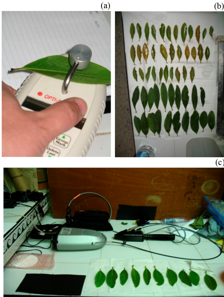
Figure 1.8: Optical CCM-200 (a), optical assessment samples of mangrove leaves (b), ASD FieldSpec HandHeld device with plantprobe (c)
