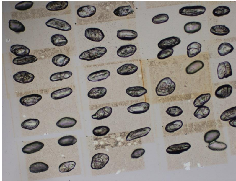
Figure 4.20 Transmitted light image of some mounted zircon grains (sample G067A1 - 10645), showing the variance in size, shape, colour, and internal zoning
