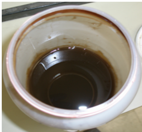
Figure A.2.1: Dispersed mixed magnetite-maghemite in electrolyte solution
