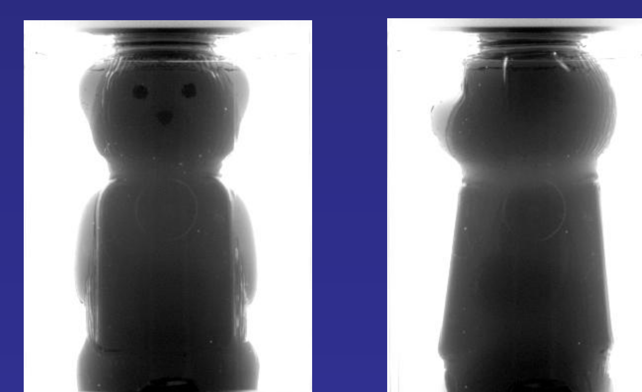
Figure 2 The BillyBee™ honey bear container is filled with blue liquid dye. Radiographic views are shown in grey-tone.
