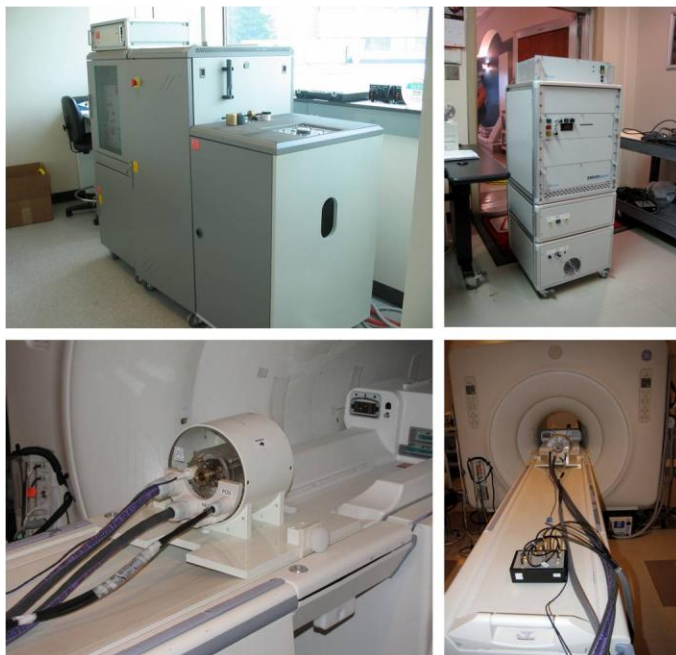
Figure 2.8 NMRD data was acquired using the Spinmaster FFC2000 1T C/DC (Stelar s.r.l., Italy) and MRIn equipment. NMRD data for magnetic field strengths ranging from 0.010 MHz to 42.49 MHz was acquired using the SpinMaster relaxometer (Top Left). Top Right and Bottom Row: The insertable field-cycling relaxometer system (MRIn, Stelar s.r.l., Italy) used to acquire NMRD curves for \pm 0.25 T field shifts about the clinical field strengths of 1.5 T (Top Right and Bottom Row).
