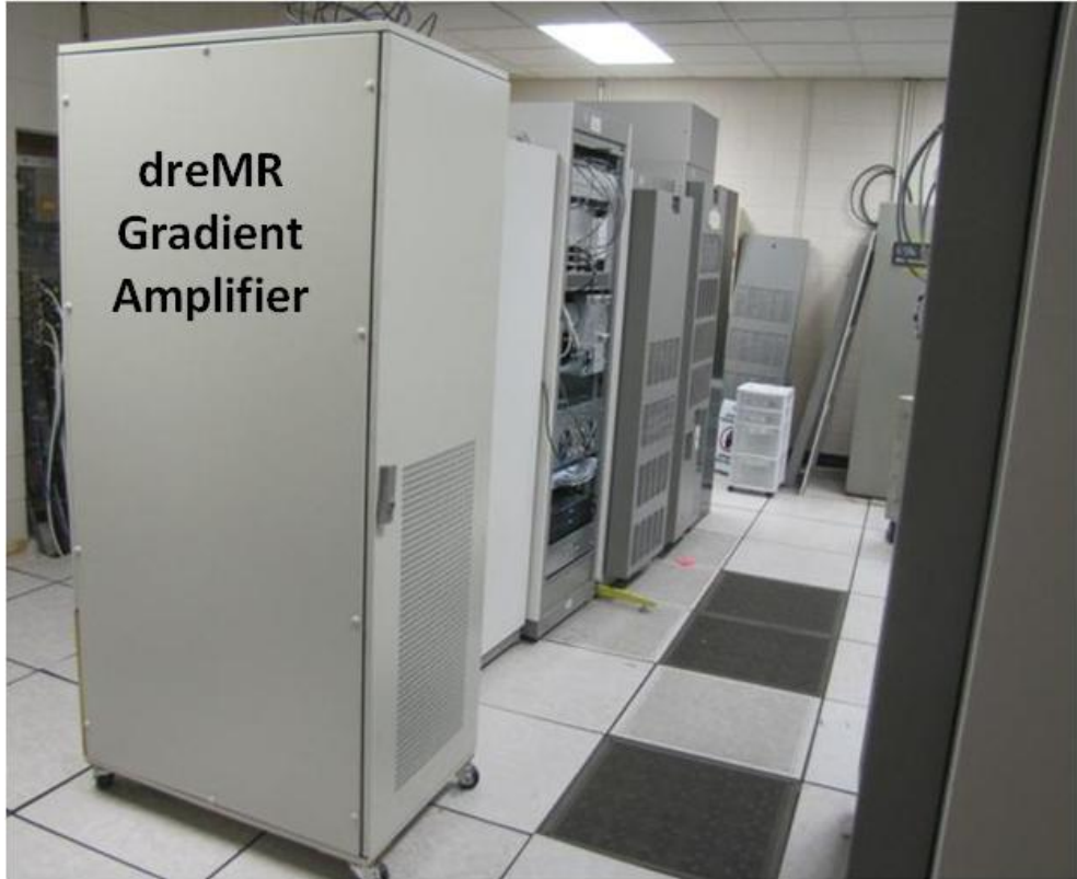
Figure 2.2 dreMR gradient amplifier positioned next to MR scanner hardware in the scanner equipment room.
