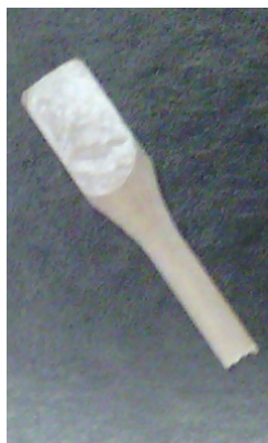
Figure 5.16 Image of nano-TiO 2 /PET with deposited stearic acid on the surface.
