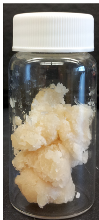
Figure 5.3 Digital picture of synthesized linear polyester from experimental section 5.2.3. Raw materials: Phthalic anhydride, adipic acid, 2,2-dimethyl-1,3-propanediol and 1,4-butanediol. Reaction took place at 165°C under nitrogen flow protection.
