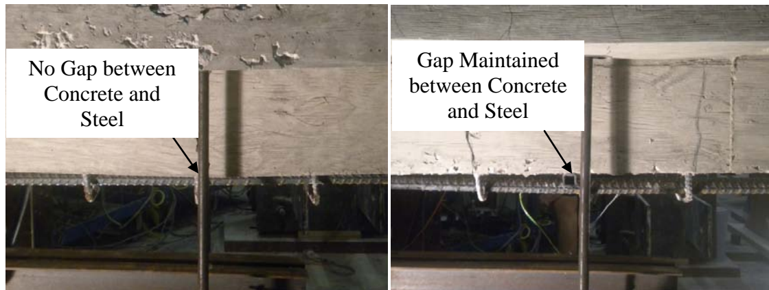
Figure 4-14: Impact of Steel Spacer under the Interior Load \omega Near the Left Support: (a) Specimen 2 and, (b) Specimen 3.
