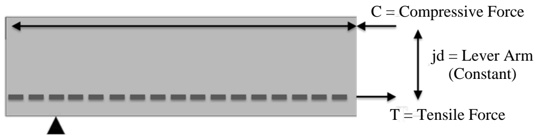
Figure 2-13: Beam Action with Constant Lever Arm if Flexural Reinforcement is Fully Bonded.
