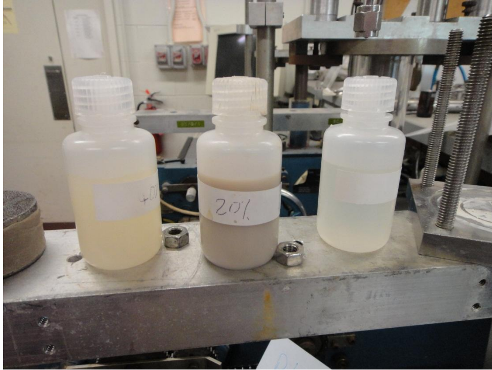
Figure 4.10: Turbidity in G80K20 effluent
