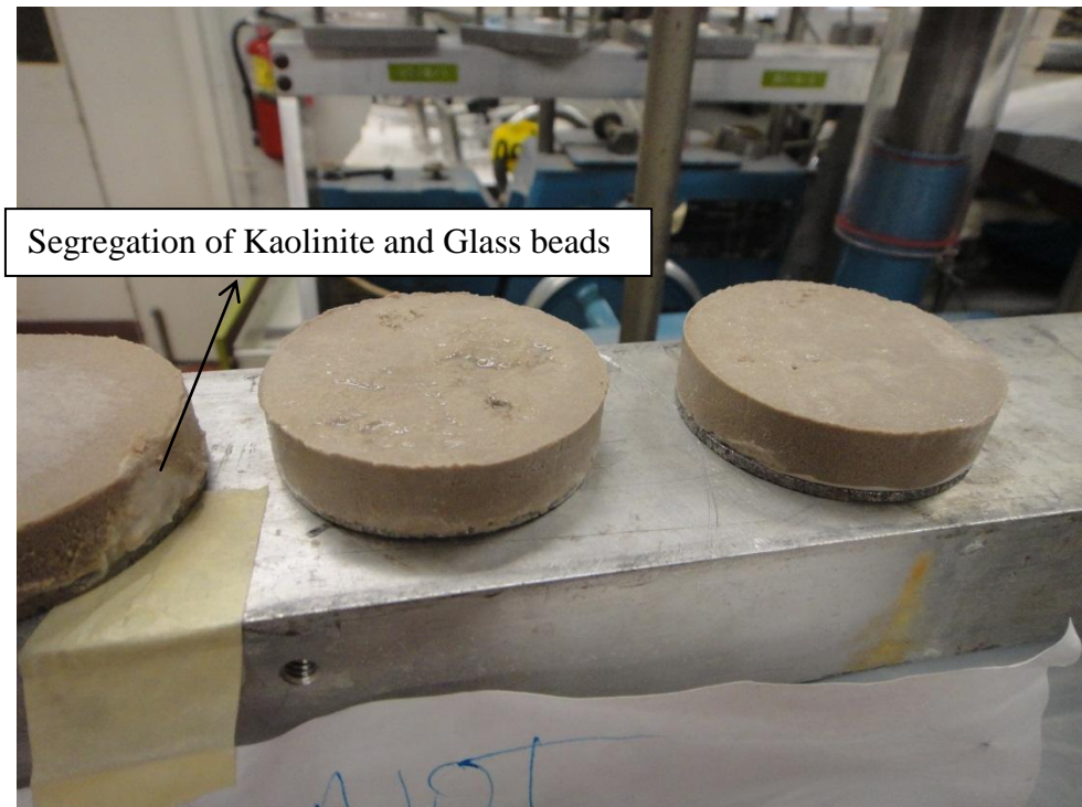
Figure 4.11: Segregation of kaolinite and glass beads in G80K20
