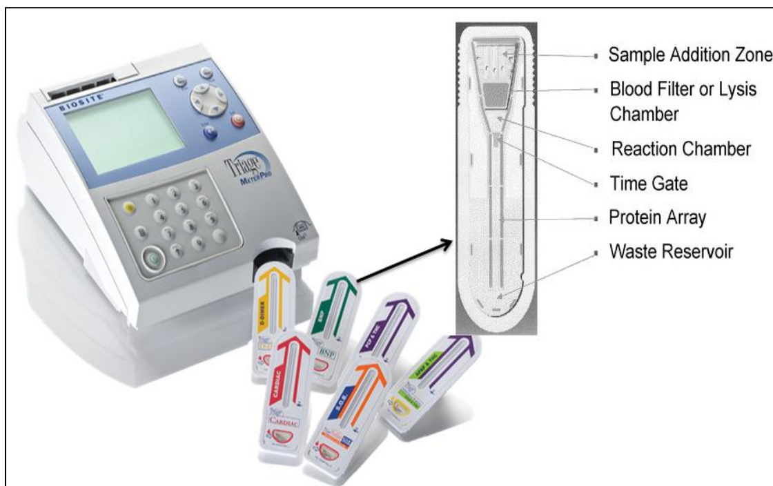
Figure 2.10: Biosite’s Triage flow-through detection technology. Reprinted with permission from Biosite.
