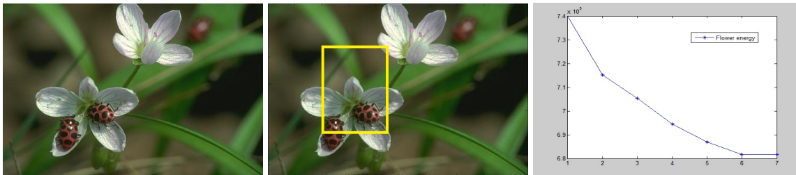
Left: original flower image, middle: foreground detection, right: the convergence process of energy
