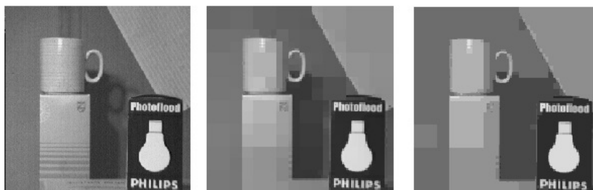
Figure 4.10: Left: original image, middle: image after quad spliding, right: image after merging 6
