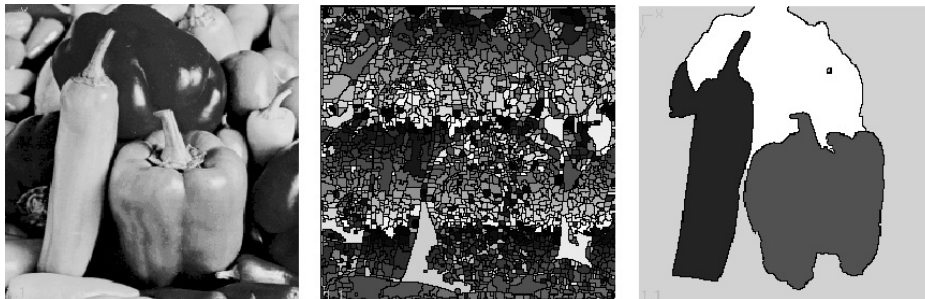
Figure 4.8: Left: original image, middle: row watershed segmentation, right: watershed segmentation using region marks to control over segmentation 4
