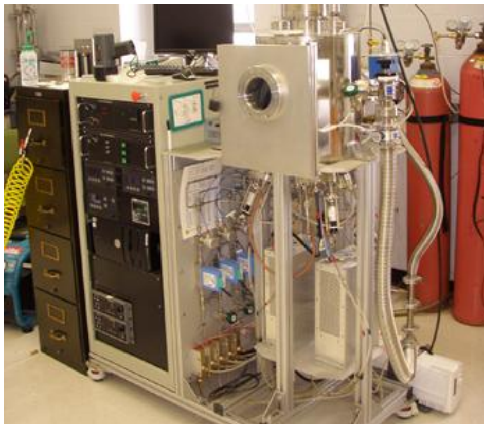
Figure 2.3 A photo of the modified PECVD/Sputtering system used for \text{TiSiO}_x coating of NCNTs.
