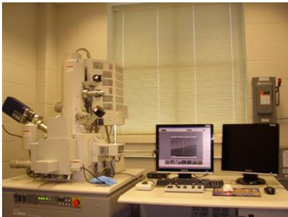
Figure 2.4 A photo of SEM (Hitachi, S-4800) machine.
