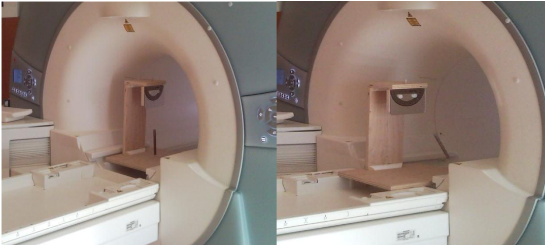
Fig 2.4: [Left] shows the deflection of 0 deg. for copper, [Right] shows a deflection of 29 deg. for stainless steel.
