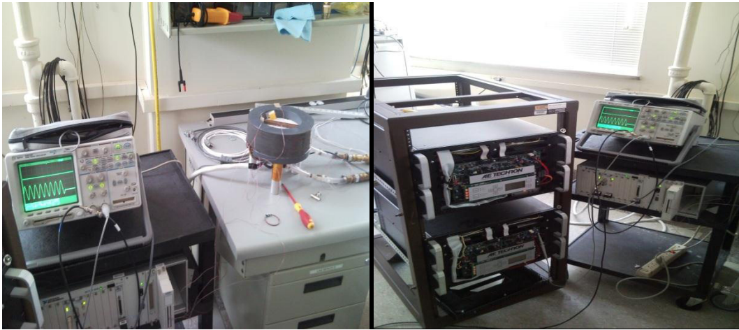
Fig. 3.5: shows the setup configuration for the gradient heating experiment with the lab magnet [left], the amplifier and acquisition system [right].
