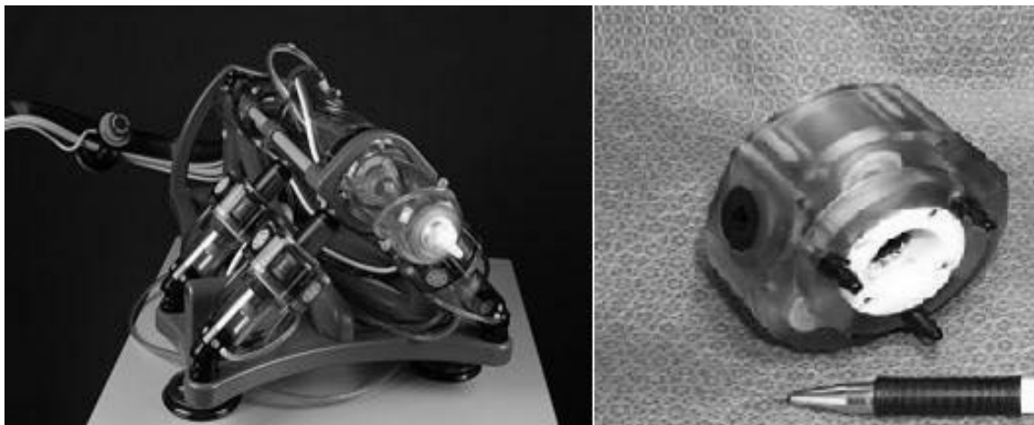
Fig.1.4: (a) The robot with six motors [21] (b) "PneuStep" the air motor [19]
