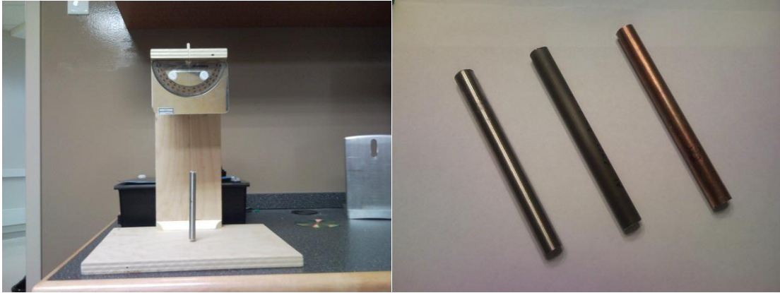
Fig. 2.3: [Left] shows the test fixture used in performing the force measurement, [Right] the shape of the test samples used in the experiment.
