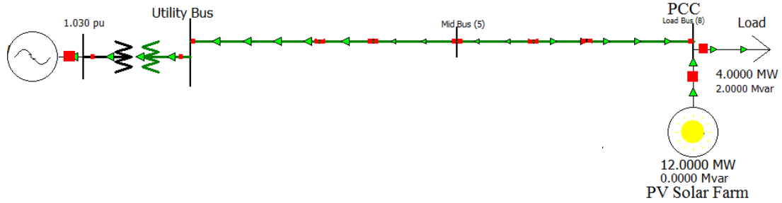
Figure 5.4 Scenario 1: PV system connected at feeder end.
