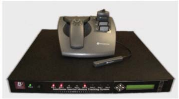
b) IS-900 ultrasonic tracking system
