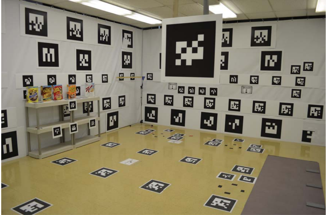
Figure 3.2 Picture showing the physical space in which installed fiducial markers in the walls and on the floor.
