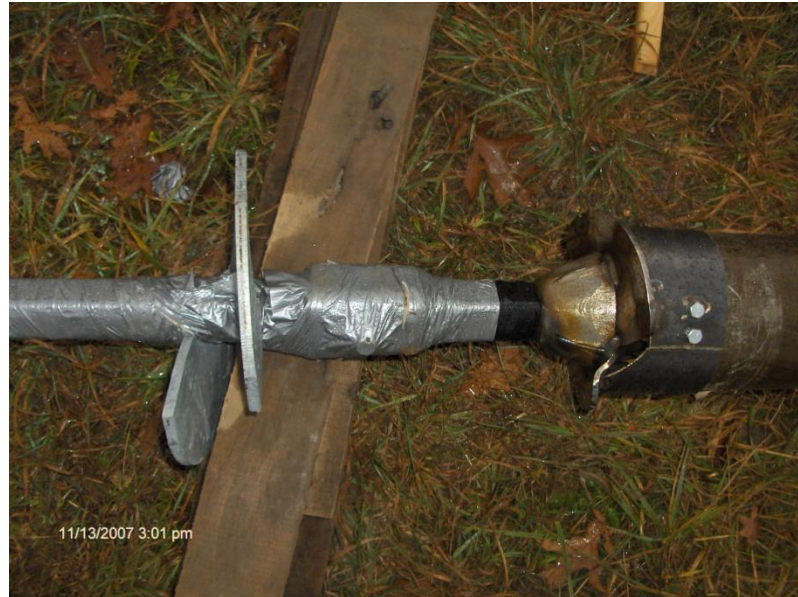
Figure 2.3. (a) Typical schematic of FRP-HPM; and (b) Cutting disk – FRP tube connection above top helix; after Abdelghany (2008).
