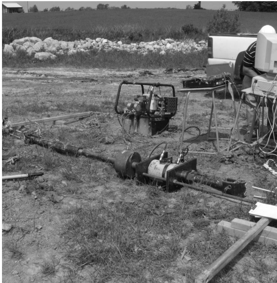
Figure 6.3. Cyclic test set-up.
