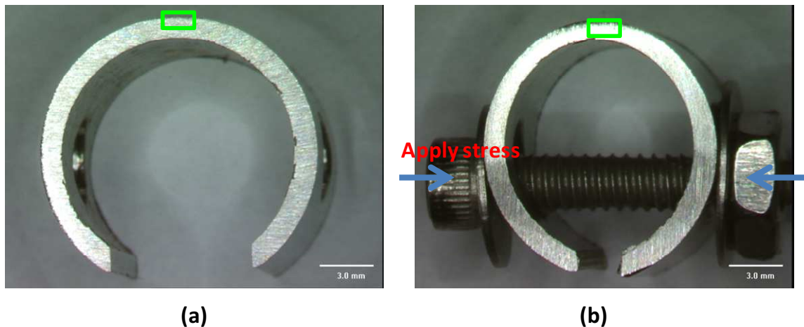
Figure 2.2 Optical images of a C-ring: (a) before and (b) after stressing by bolt tightening to achieve a nominal 2% strain. Green boxes at the sample apex indicate the analysis area.
