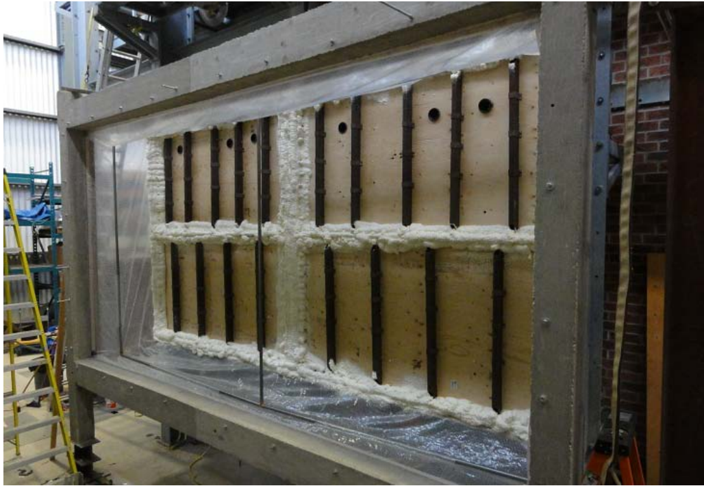
Figure 3-19 - As-built Concrete Frame with Airbag and Back Panel
