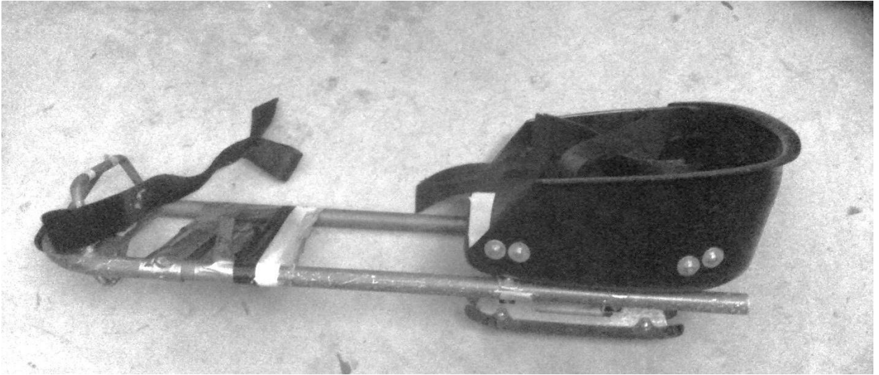
Figure 5: An earlier sledge design consisting of rails, seat, a nose, and skate blades.
