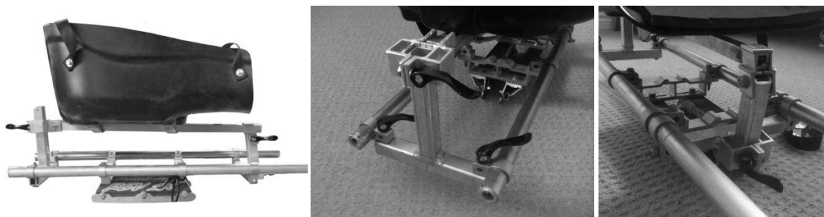
Figure 20: Pictures of the side, back, and front of the adjustable test sledge used in this study. The quick release collars (black levers) allow the seat to be vertically and horizontally adjusted with ease as compared to using bolts.
