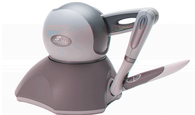
Figure 6.1: The PHANTOM Omni haptic device (from http://www.sensable.com/ )
