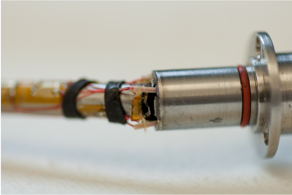
Figure 4.12: Broken weld lines on middle shaft.
