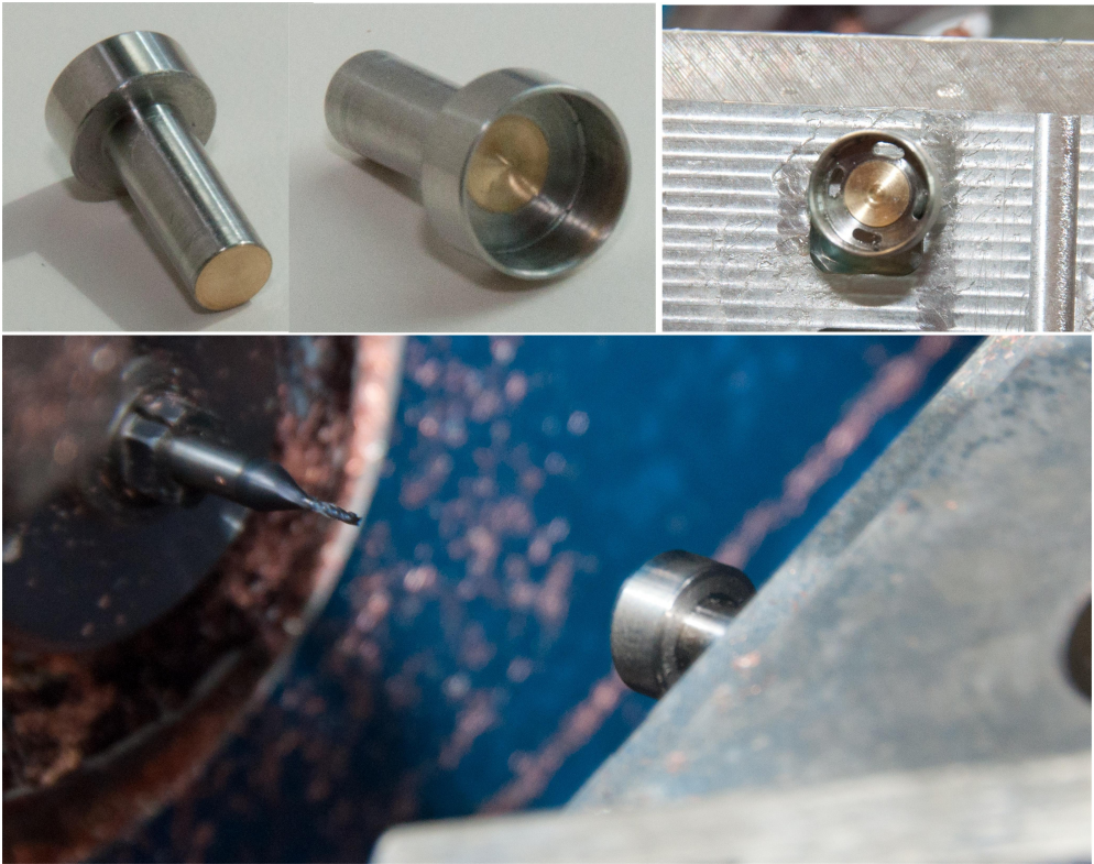
Figure 4.15: Mounting of axial element on MMC: axial element with brass dowel ( top left ), element mounted on MMC during drilling of small slots ( bottom ), and element mounted on MMC after machining ( top right ).
