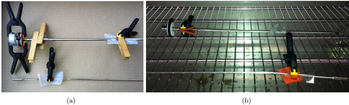
Figure 5.5: Strain gauge installation process: gauges clamped for curing (a) and instruments in oven (b).
