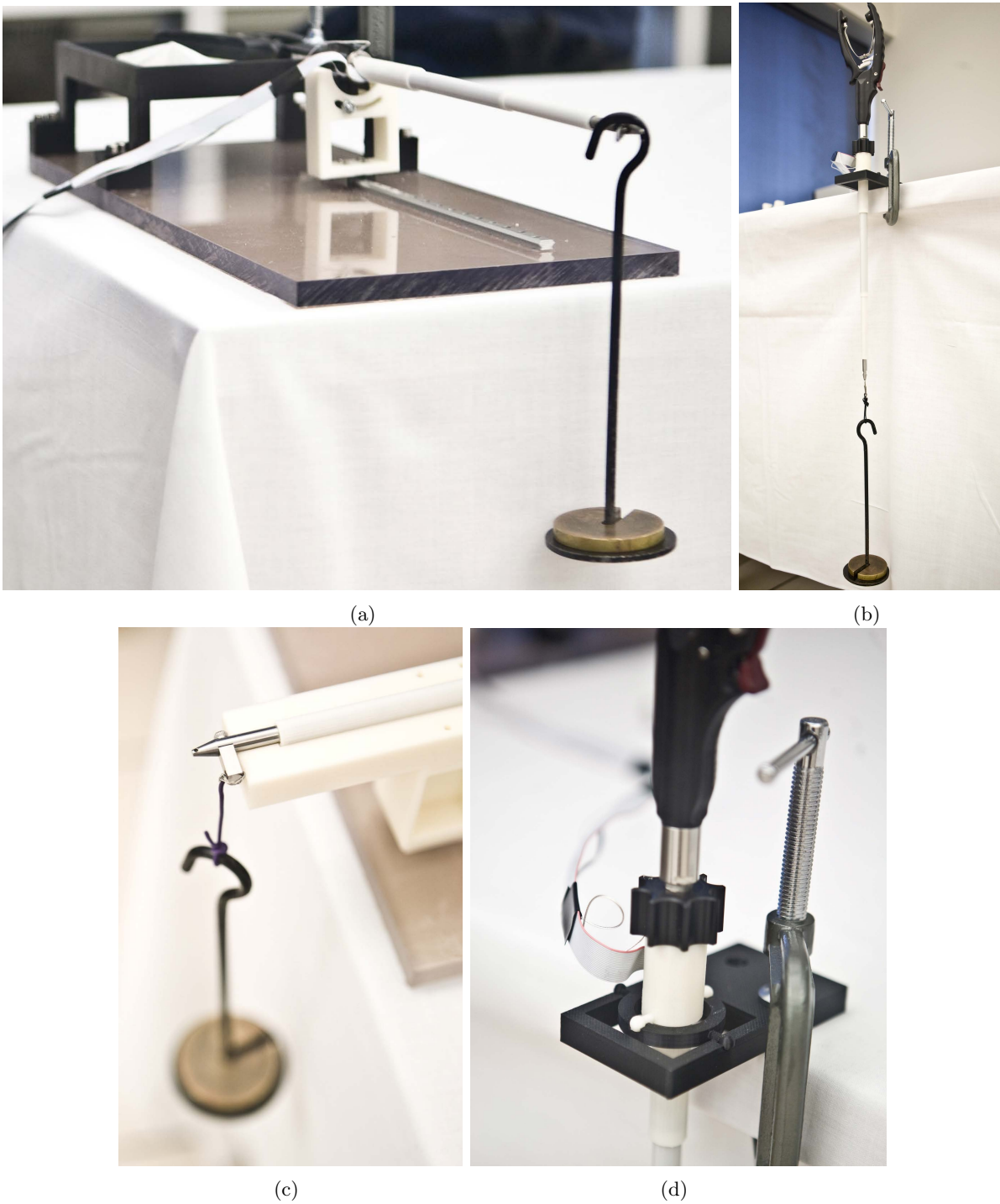
Figure 3.12: Instrument placement for calibration for: x and y moments (a), axial (b); and torsion (c). (d) Shows a close up of the gimbal designed for the application of axial forces. Note that in these pictures, the stainless steel outer shaft was replaced by an ABS plastic shaft. Photo credit: Meg Woodhouse.
