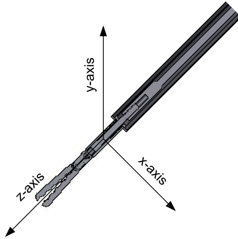
Figure 3.3: Coordinate frame associated with the instrument.
