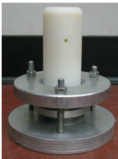
(b) Assembled compaction cell
