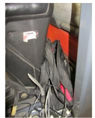
Figure 9 - Bag used to store dataloggers behind operator's seat during testing
