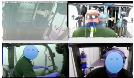
Figure 7 - View of synchronized videos in a 2 by 2 arrangement. The top left view is from the eye gaze camera on the goggles; the top right from the camera at the back; bottom left from the camera at the side; bottom right is from the camera at the front of the forklift.
