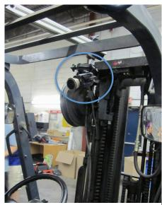
Figure 5 - Camera at the front of the forklift.
