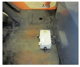
Figure 7 - IMU magnetically attached to the forklift chassis at the base of the seat
