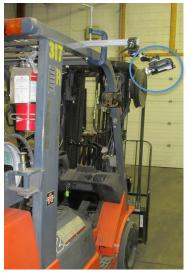
Figure 4 – Camera on lateral side of the forklift
