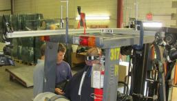
Figure 3 - View of custom-made cross on top of the forklift attached with cclamps
