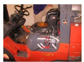
Figure 5 - View of IMU underneath rubber mold on the seatpan and cables secured to the chassis, leading into bag behind operator's seat
