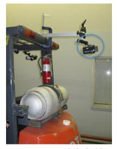
Figure 6 - Camera at the back of the forklift.
