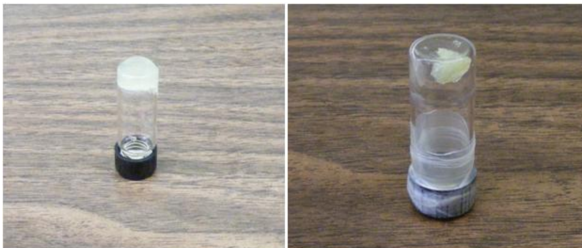
Figure 2.16: Picture display of polymeric nature of complex 2.13 . (Left) solvent acetone. (Right) solvent DCM.
