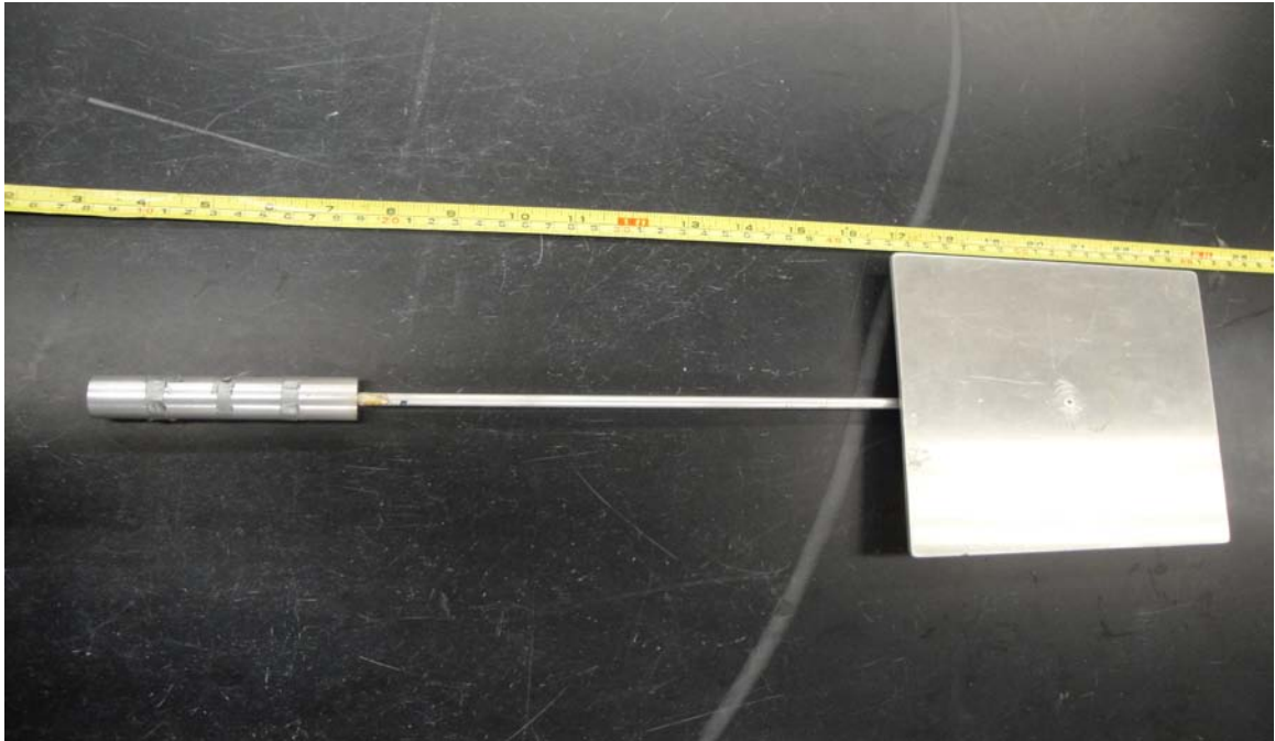
Figure B-3. Pile, Pole, Plate Model
