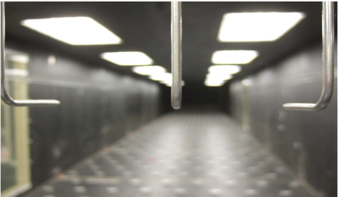
Figure B-10. Reference Pitots in Wind Tunnel Testing
