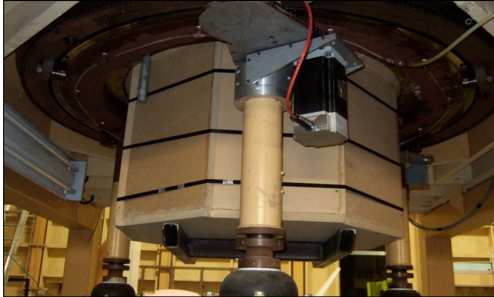
Figure 3-6. Supporting System of the Wind Tunnel Sand Box
