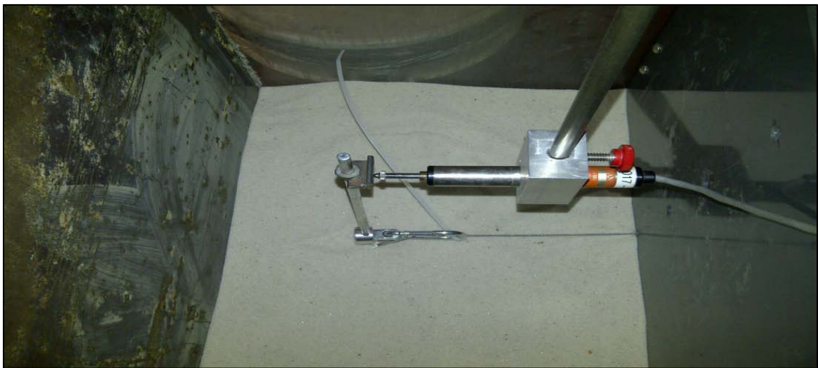
Figure 3-17. Static Ground-line Test
