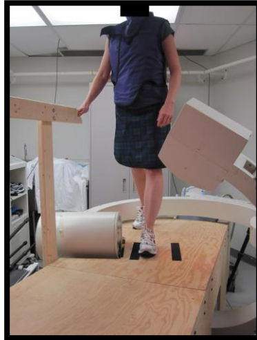
Figure 5.1: Platform and wrap-around leaded clothing.
