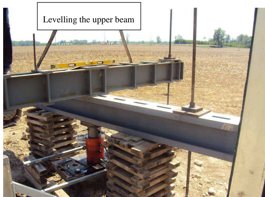
Figure 6. 5. Centering and leveling the upper beam over the lower one
