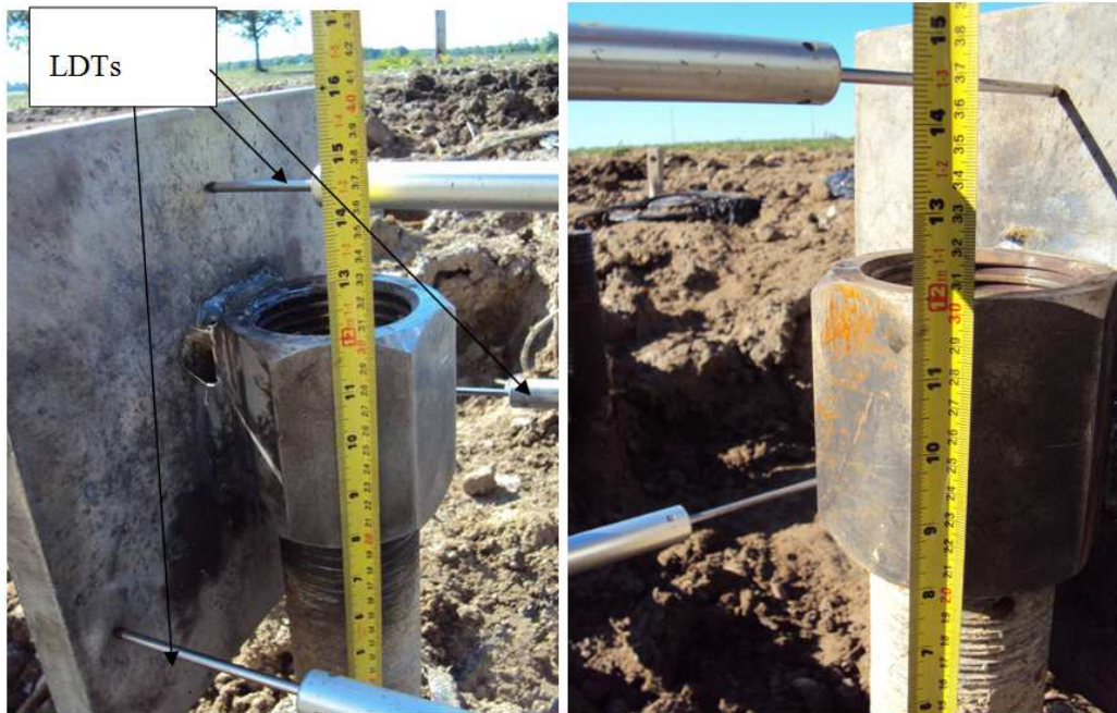
Figure 7. 3. Position of the applied load during the monotonic lateral tests
