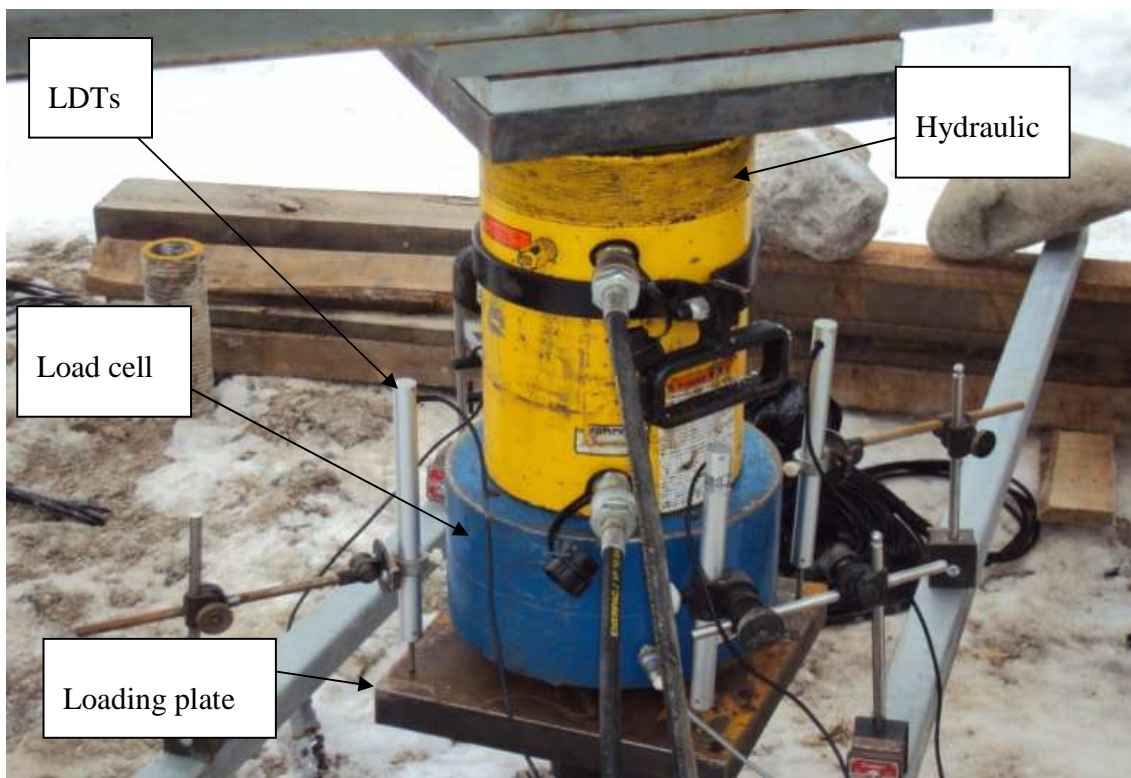
Figure 5. 4. Micropile head instrumentation during compression tests
