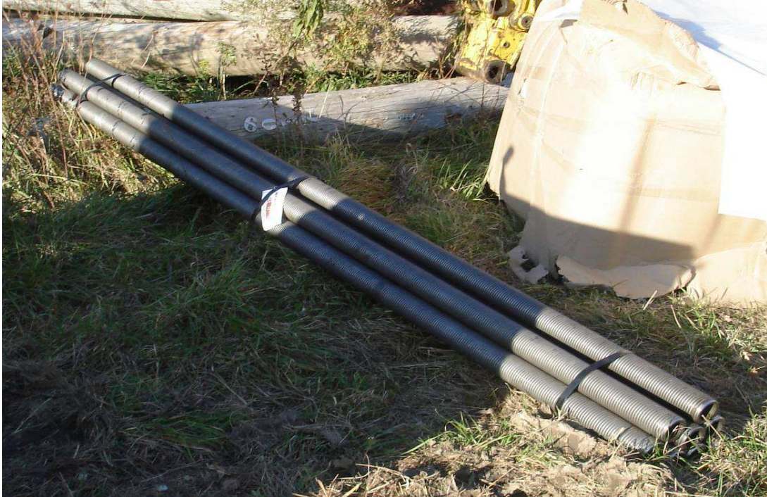
Figure 4. 6. B7X1-76 Geo-drilled hollow core bars
