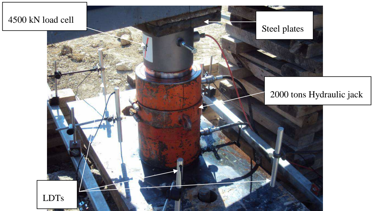
Figure 6. 7. Arrangements of the instruments at the top of the steel pile raft
