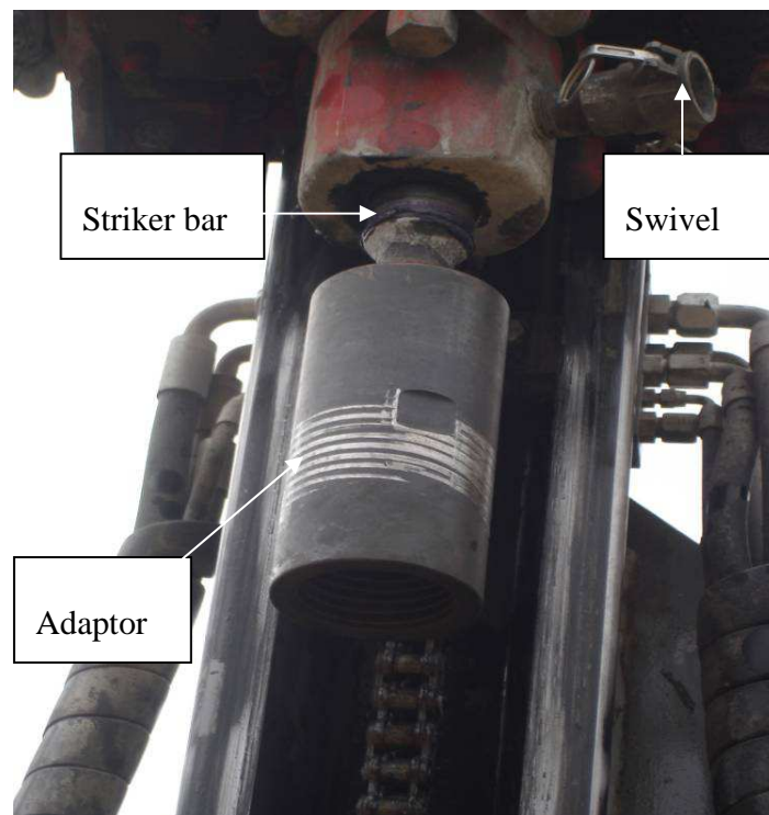
Figure 4. 9. Final connections at the top of the drifter
