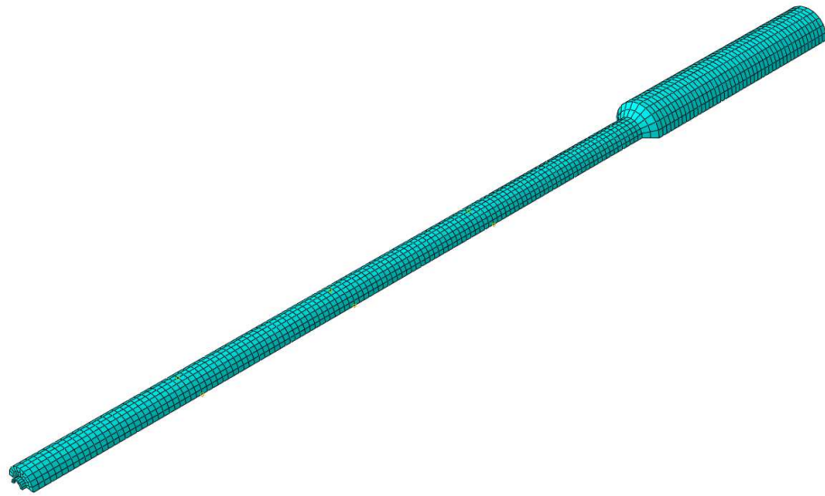
Figure 6. 18. The geometric model of the micropile in the group analysis
