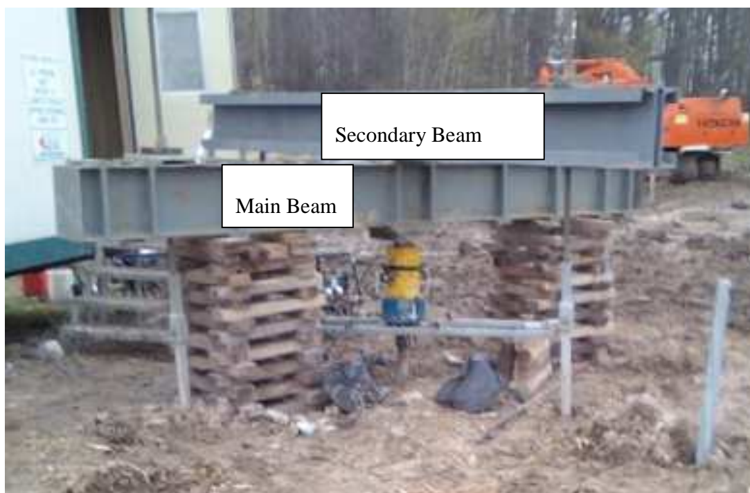
Figure 5. 2. Reaction frame used during monotonic and cyclic loading
