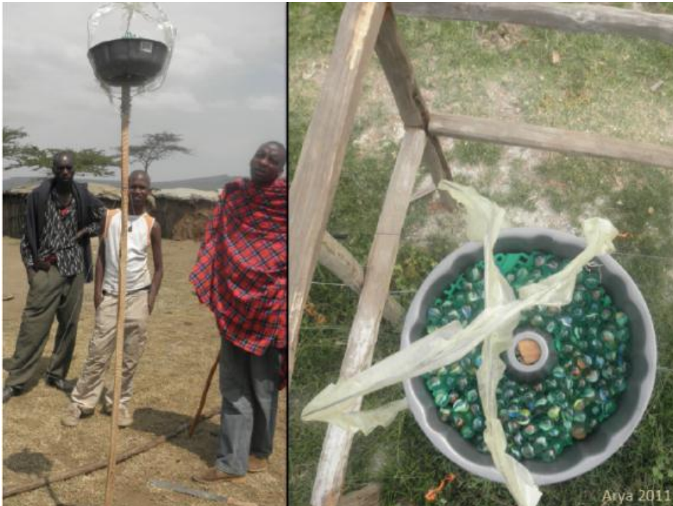
Figure 2.3: Apparatus used for dust collection. On the right is an overhead photo of the dust collector. On the left is a profile shot, showing relative height from the ground.
