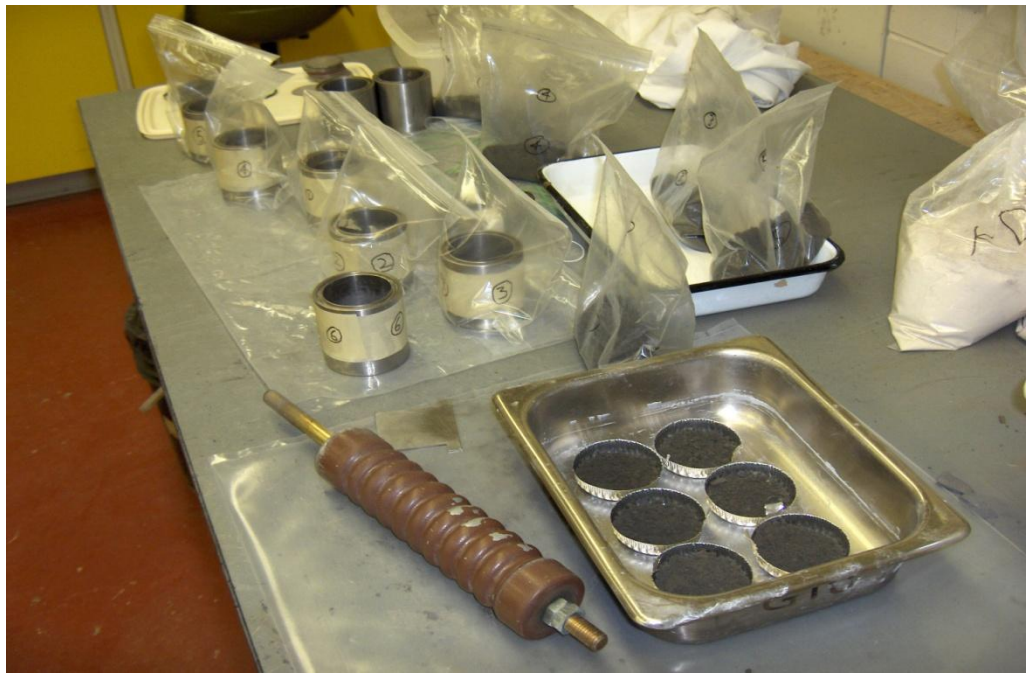
B.2 Casting of cemented paste tailings samples for saturated hydraulic conductivity tests
