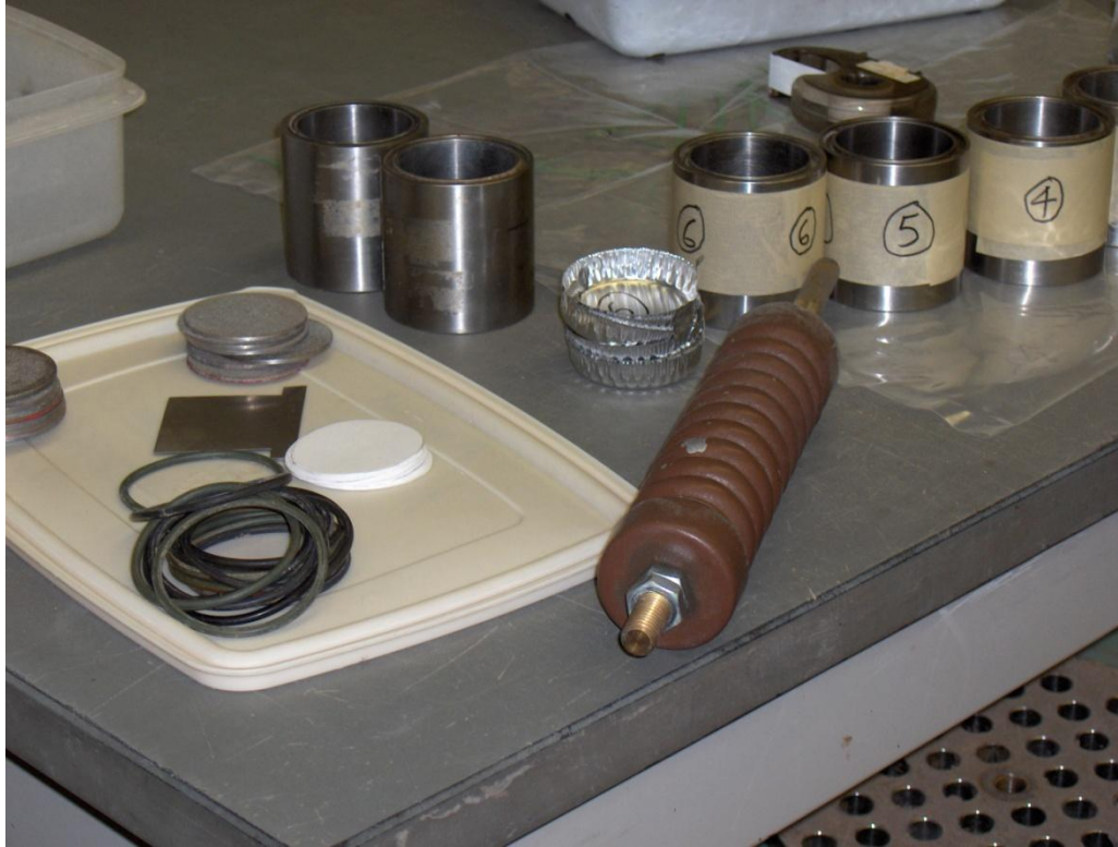
B.1 Steel cylinders with porous disks and rubber rings for saturated hydraulic conductivity tests
