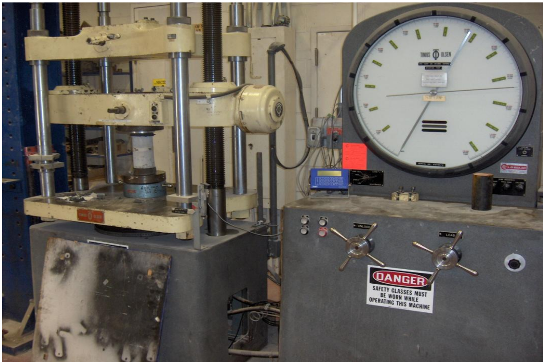
A.6 Super 'L' Tinius Olsen Universal Testing Machine (UTM) for UCS tests
