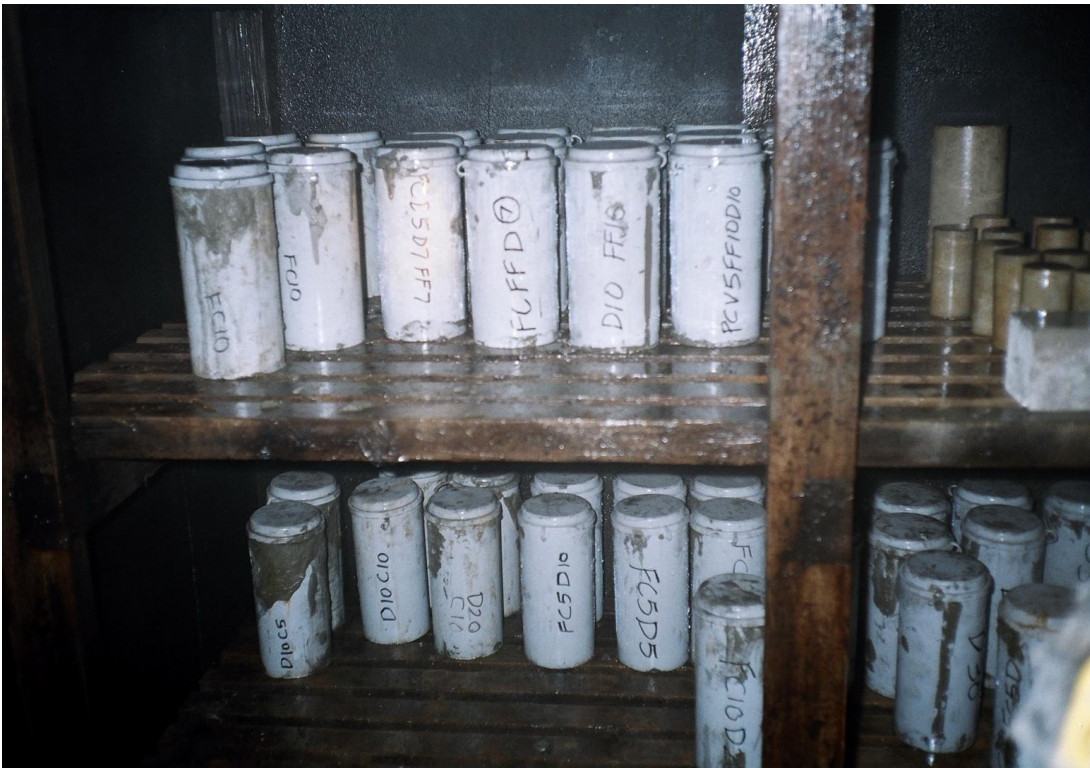
A.4 Mine tailings samples in humidity chamber for curing under controlled conditions
