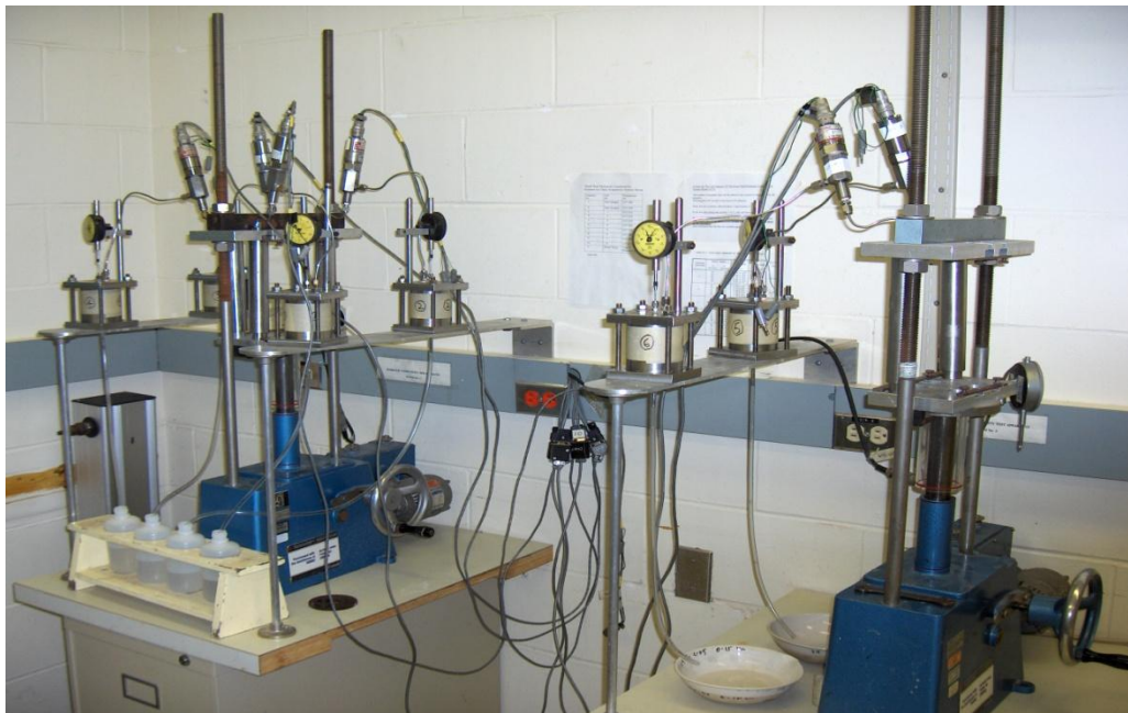
B.3 Fixed wall constant flow rate hydraulic conductivity apparatus for measurement of saturated hydraulic conductivity of cured cemented paste tailings samples
