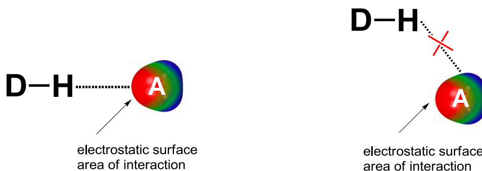
Figure 1-6 Hydrogen bonding between the acceptor (A) and the hydrogen atom of the donor (D). The directionality of the (head-on or end-on binding, not side-on binding) electrostatic surface dictates the directionality of the hydrogen bonding which is not observed on the right resulting from an acute bond angle and where there is no contact with the electrostatic potential area of interaction (shown in red in potential map).
