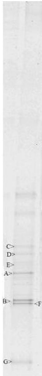
Figure 3.6 - DGGE profile of the 16S rDNA gene fragments for the AADS [Hafez et al., 2010a]
