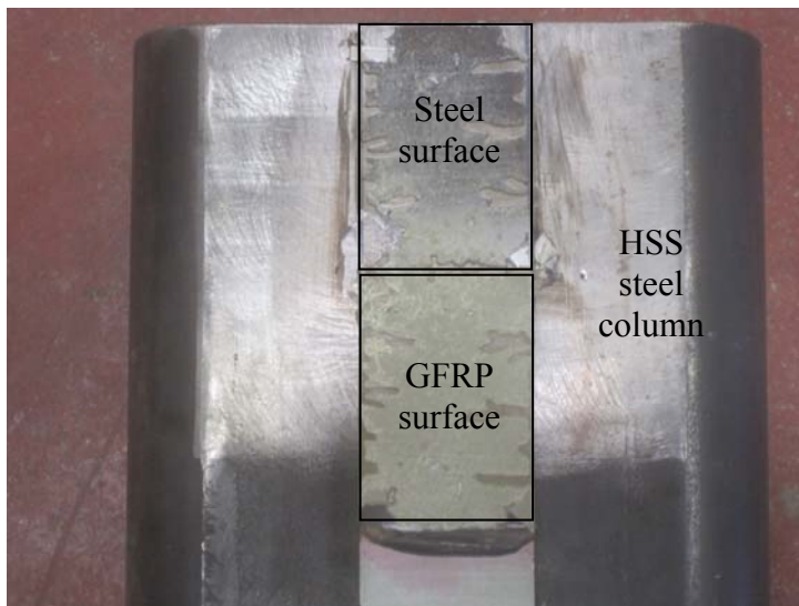
Figure 5.5 A photo of a mode of failure of the adhesive.
