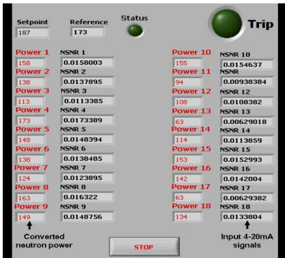
Figure 6.7 – Real-time monitoring interface
