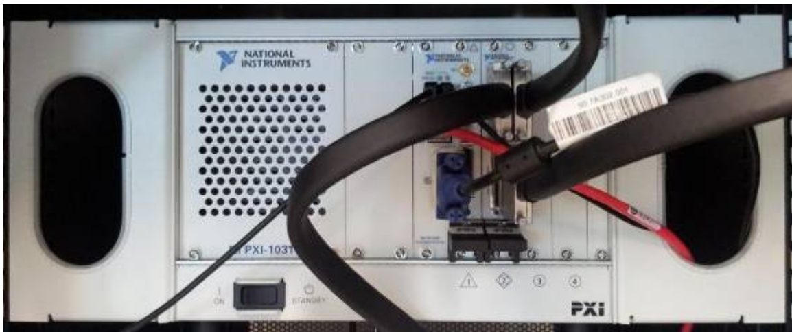
Figure 6.2 – National Instruments PXI-7811R FPGA platform
