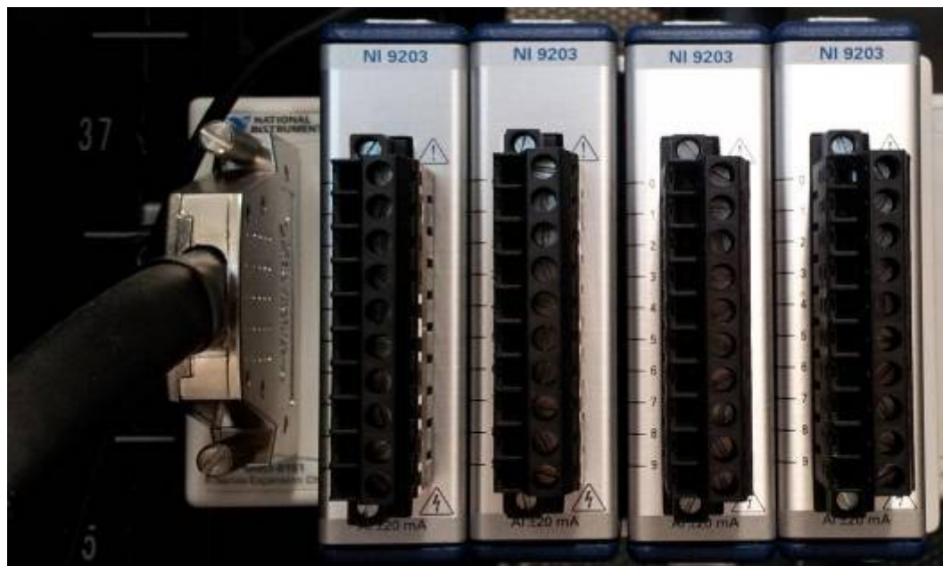
Figure 6.3 – National Instruments expansion chassis and I/O modules
