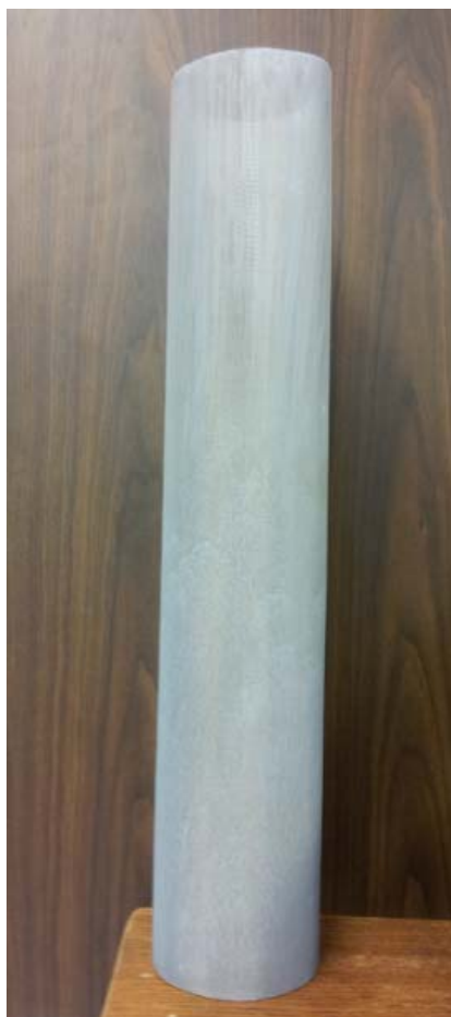
Figure 14: Stainless steel mesh cylinder coated with Degussa P25.
