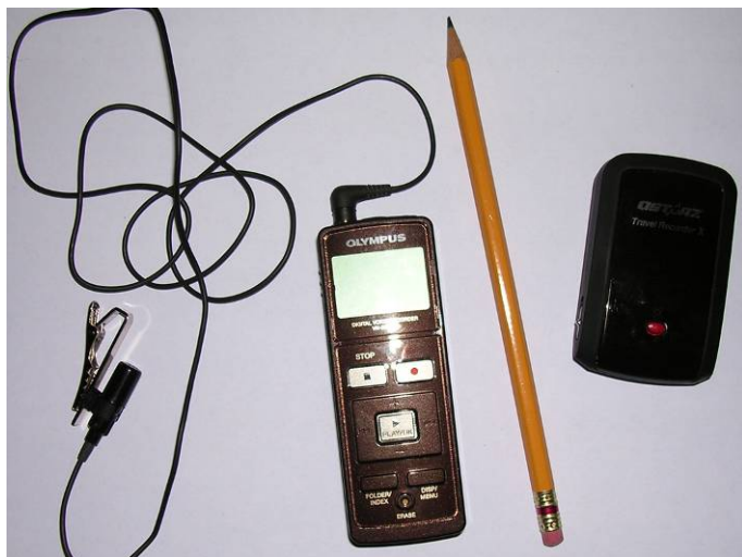
Olympus ME15 lapel (lavalier) microphone, Olympus VN-5200 PC digital voice recorder, and Qstarz BT-Q1000X GPS data logger. Not shown: Crown Sound Grabber II PZM Microphone (for interviews).
