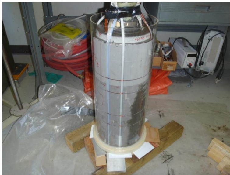
Figure 4.10: A photograph of the basic potting procedure for each layer. A mould was constructed from a plastic cylinder and masking tape and the epoxy was simply poured in and left to set.
