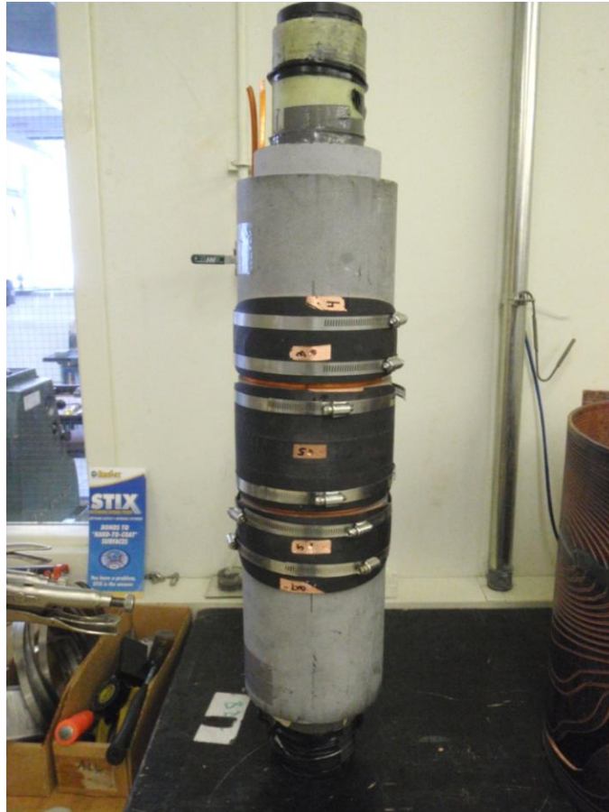
Figure 4.8: A photograph of the xz -shim coil being fastened to the insert coil. Hose clamps were used to squeeze the coil and remove flat spots resulting from the rolling procedure. Connection leads are not yet present.
