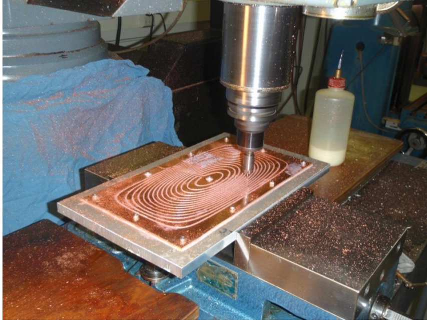
Figure 4.6: A photograph of a thumbprint of the xz -shim being milled by the CNC mill. The simulated wire patterns are fed directly into MasterCam X5 ® , the software that controls the end mill.
