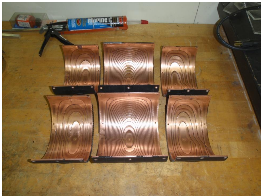
Figure 4.7: A photograph of the xz -shim coil after it had been rolled to radius. The 1.0 cm border is cut off before it is attached to the insert coil and wired together.
