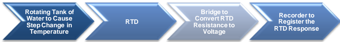
(a) Rotating Tank for Plunge Testing of RTDs
