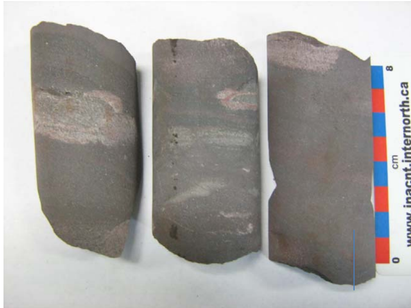
Plate 3.12: Representative samples of the Upper GIF Facies in drill core. Note the lack of chert bands and laminations.
