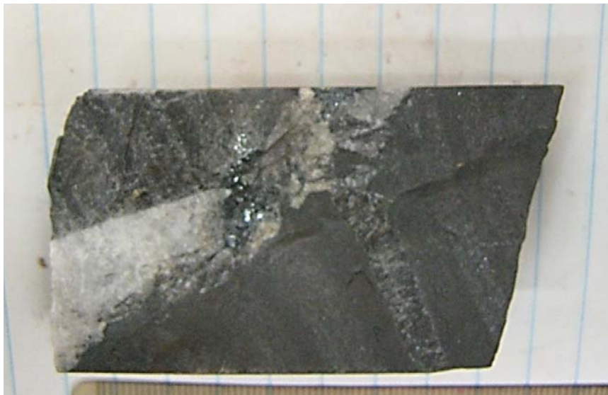
Plate 3.19: Sample 26-75-1066 showing coarse specular hematite within a late quartz vein.
