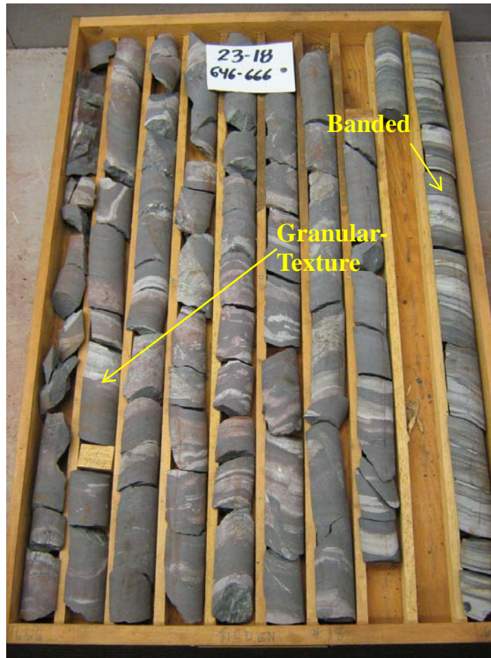
Plate 3.4: Drill core from hole 23-18-(646-666) depicting granular-textured bands interbeds within the Medial BIF Facies.
