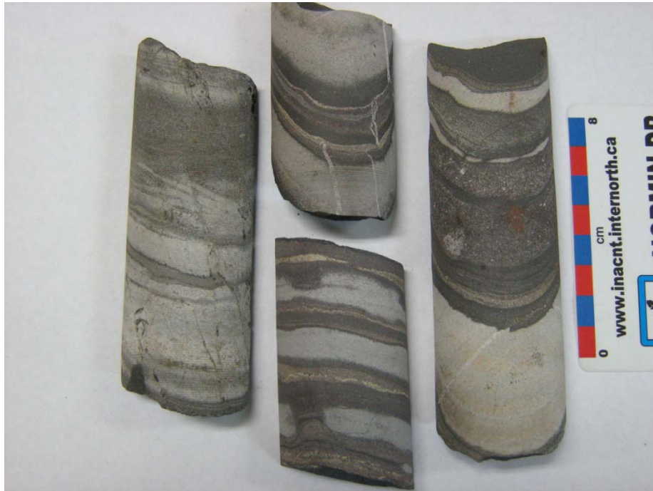
Plate 3.5: Representative samples of the Medial BIF facies. Band lithologies are: white cryptocrystalline chert, yellow carbonate, black oxides, pinkish granular-chert and speckled clastics. Note that there are multiple fractures and offsets that cross-cut banding.
