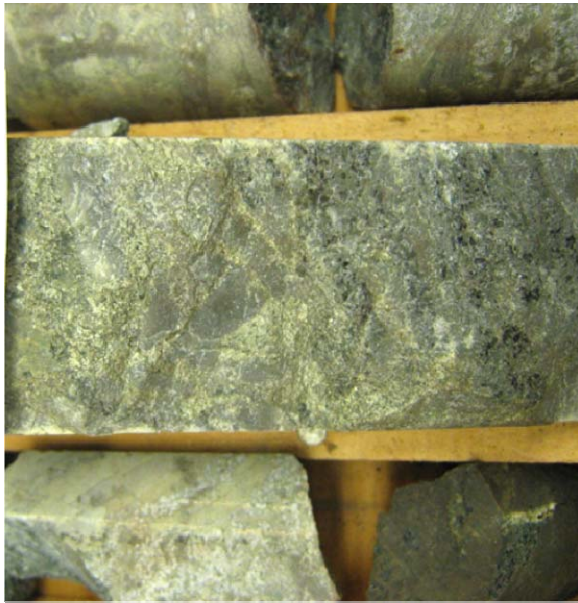
Plate 3.18: Sample 26-77-1157 depicting late sulphides infilling fractures within the Basal Clastics.
