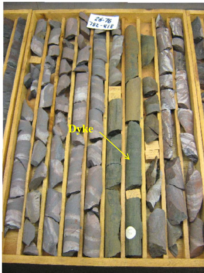
Plate 3.15: A chloritized dyke intruding the Upper GIF Facies in drill hole 26-076 (782-818).
