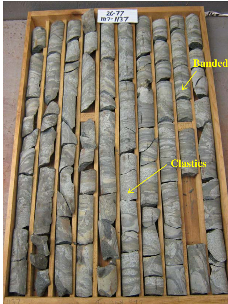
Plate 3.0: Drill core of hole 26-77- (1117-1137) depicting coarse clastics interbedded with Medial BIF at the base of the Main Pit Carbonate Domain.
