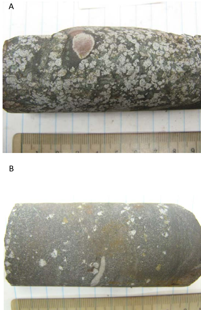
Plate 3.1: Clastic lithofacies: (a) coarse clastics (sample 23-70-1113); and (b) fine grained variety (sample 26-70-1236).
