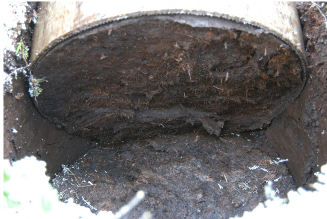
Figure A4. The core bottom being detached from the permafrost at the time of sample uplifting once the core was fully sampled.
