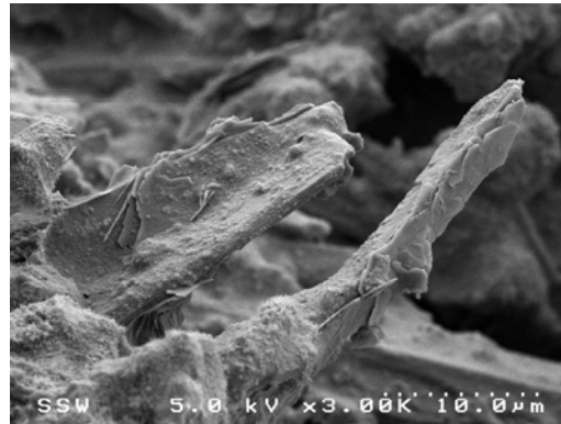
Figure 9-8: SEM for wollastonite microfibers pullout from cementitious matrix incorporating SRA.
