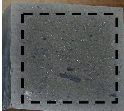
Figure 4-9: Cross section for SRA specimen exposed to drying condition after 7 days.
