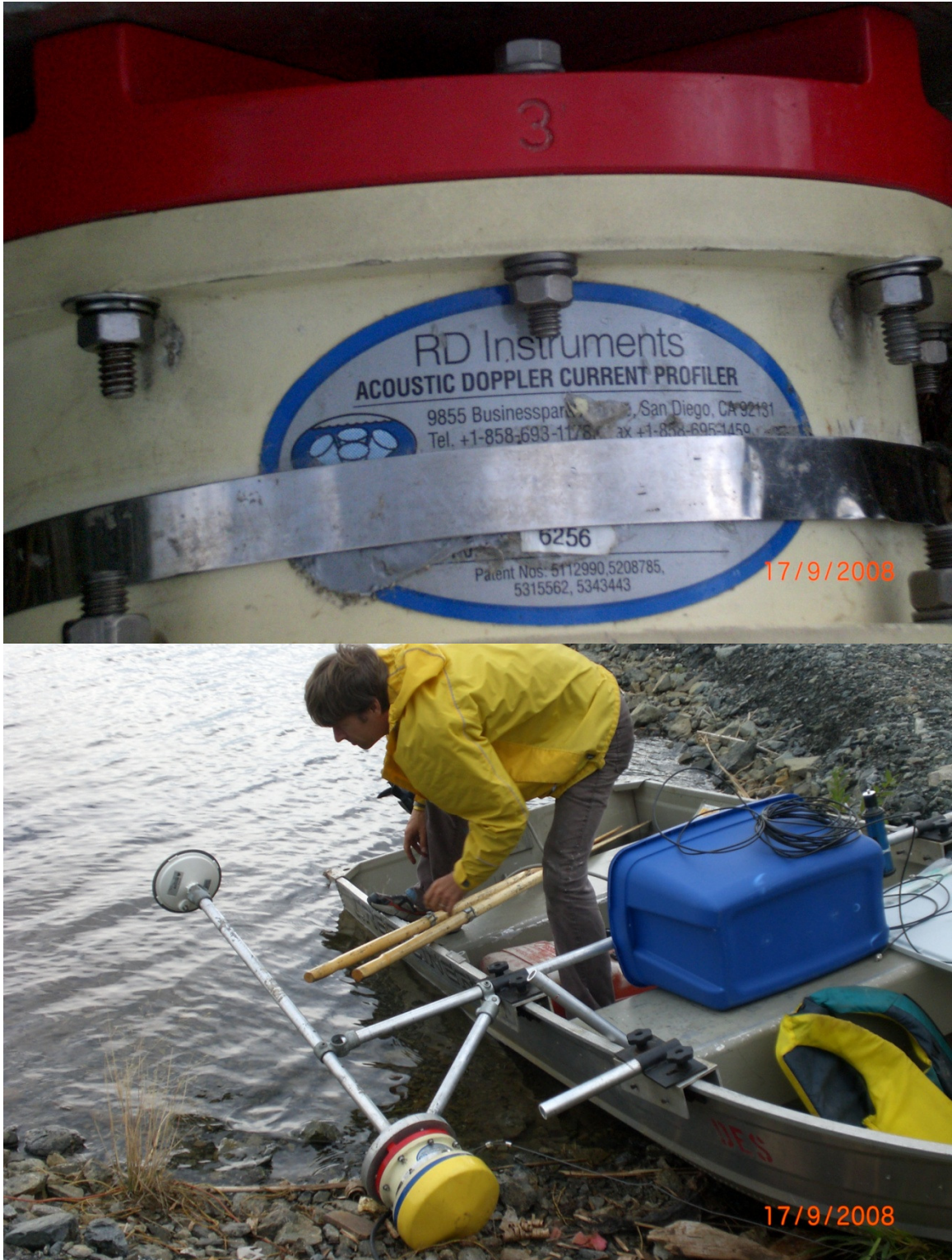
Figure IV-10 ADCP and GPS mounted on the boat with especially fabricated mounting assembly
