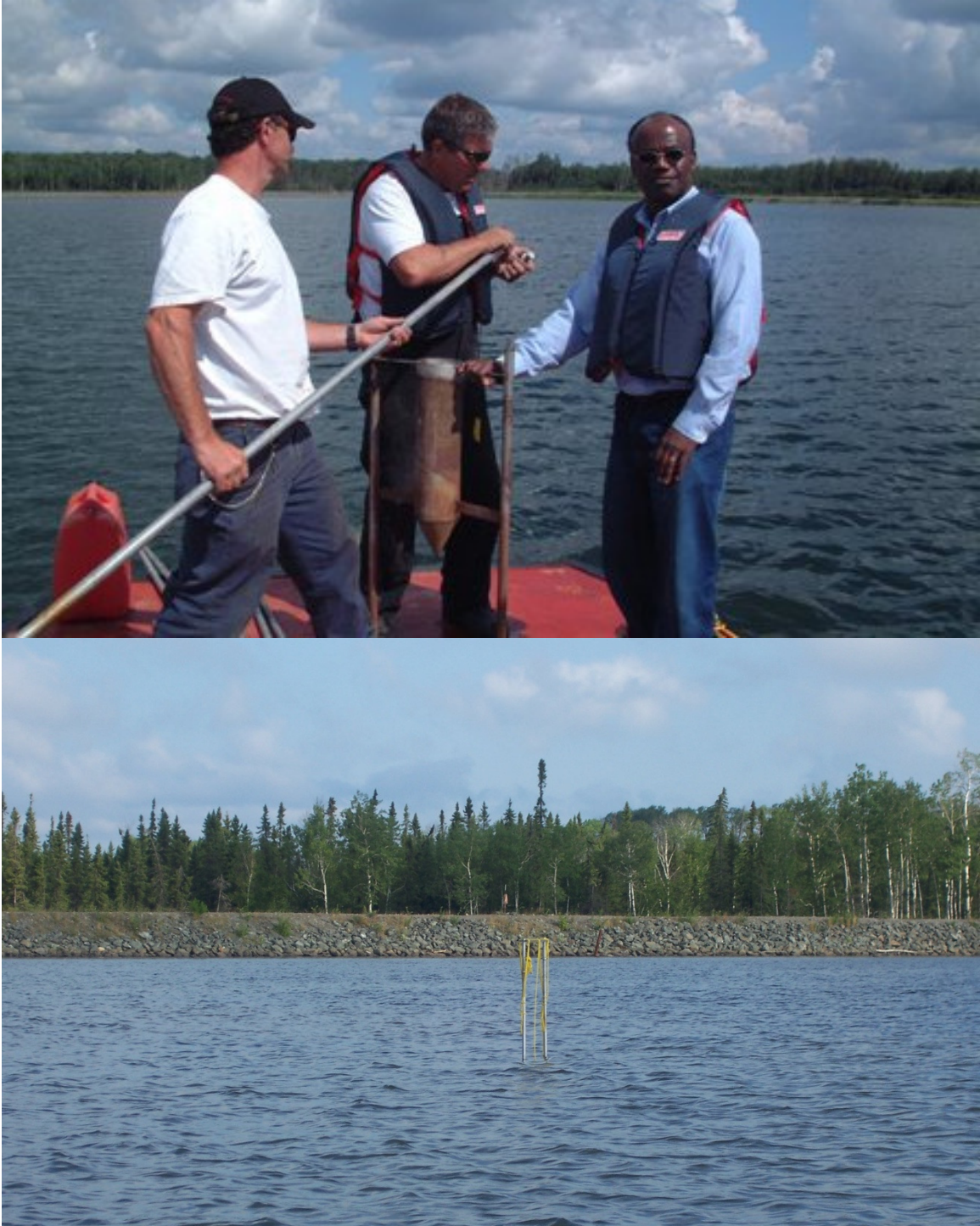
Figure IV-6 Deployment of sediment traps by professional divers under supervision of Prof. Ernest K. Yanful (on right) and a properly installed sediment trap
