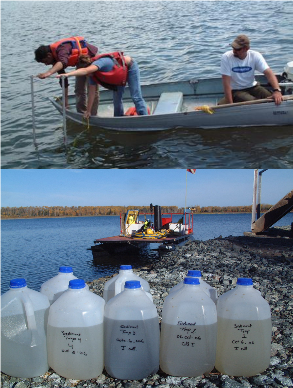
Figure IV-7 Sampling process of the sediment traps and samples collected from each sediment trap stored in 4 liter containers
