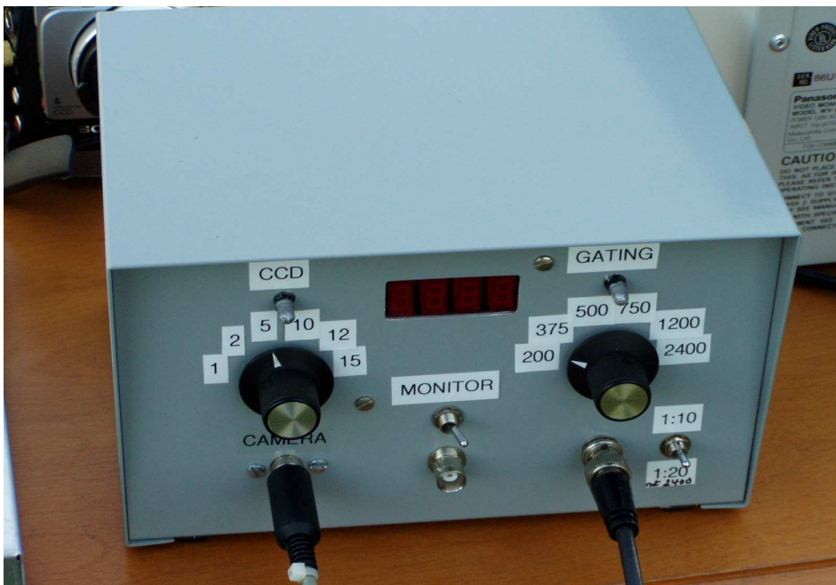
Figure 2.7: External box which controls the rate of the CCD exposure and the gating system frequency.
