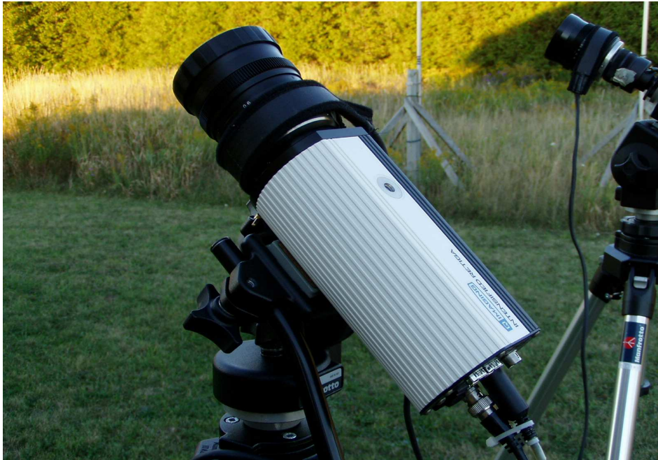
Figure 2.6: The QImaging Intensified Retiga (model 1394) electronically gated image intensified camera.
