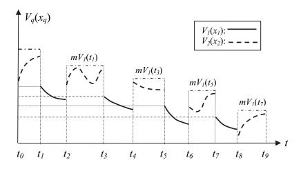
Figure 3.5: Multiple Lyapunov functions stability
