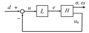
Figure 2.1: Block diagram of an internal model principle control system
