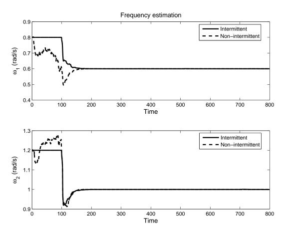
Figure 4.6: Frequency estimation using adaptive IMP algorithm
