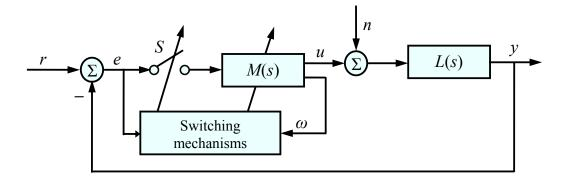
Figure 4.1: Block diagram of open and closed-loop control system
