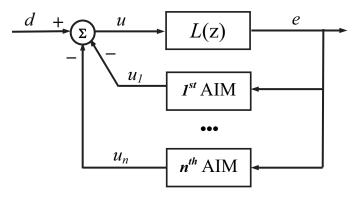
Figure 2.3: Block diagram of an adaptive IMP feedback control system for multi-EDS signals
