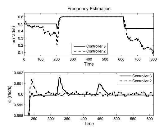
Figure 4.3: Frequency estimation of the intermittent and non-intermittent control at its initial value 0.5 rad/s. When the monitored signal  $x_m(t)$  is greater than the threshold  $x_u$  after the sinusoid is introduced at t = 199, the IMP controller is turned on by setting f(t) = 1. The adaptation of the disturbance frequency starts. In the mean time, the plant output starts to track the sinusoidal disturbance.
