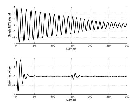
Figure 2.4: Single EDS signal with a parameter step change and error response period. From sample point 50 to sample point 150, the measurements are  $var(\sigma) = 7.7 \times 10^{-8}$ ,  $var(\omega) = 1.8 \times 10^{-7}$ .
