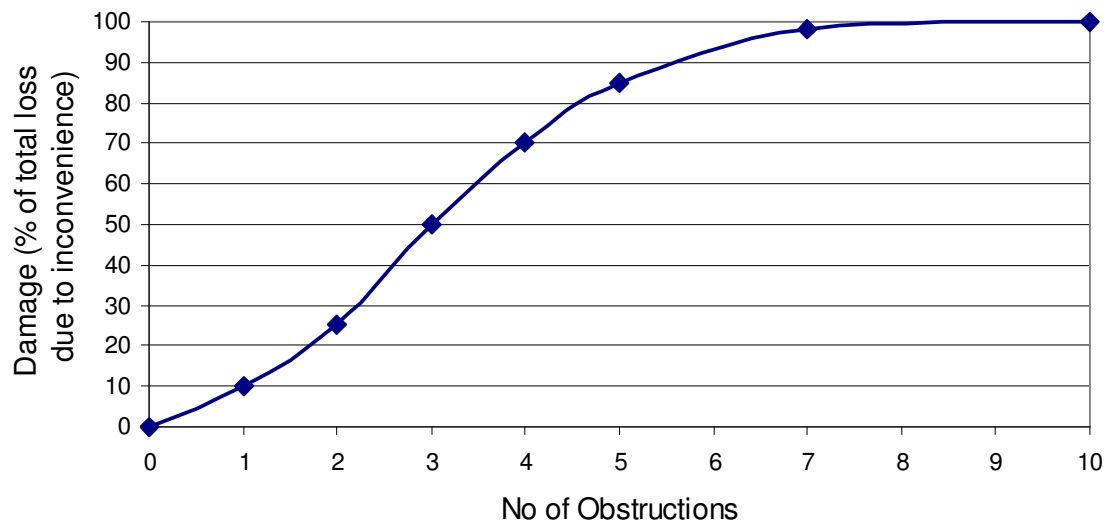
Figure 4.28: Road blockage vs. percent damage relationship
