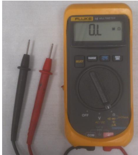
Figure 2.16: A Fluke 16 multimeter which was used to determine if a short-circuit existed in the stainless steel and silicon probes.
