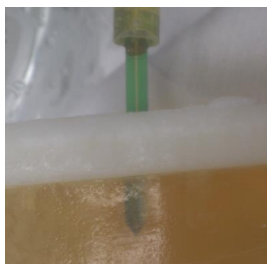
Figure 2.32: A silicon probe inserted in to the gelatine (orange) and lard (white) model during the electrical impedance testing.
