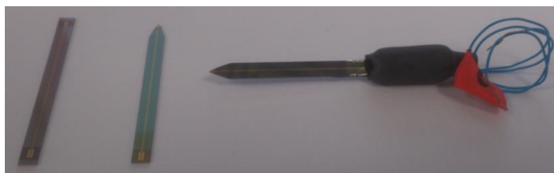
Figure 2.20: The stages of the device packaging process including diced, shaped and electrically packaged.
