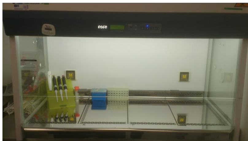
Figure 3.2: The Class II biological safety cabinet in the Tissue Culture Facility in Tyndall National Institute.
