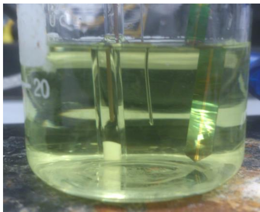
Figure 2.18: The Ag/AgCl and platinum wire electrodes and a silicon probe in a solution of potassium ferri/ferrocyanide and KCl during CV measurement.
