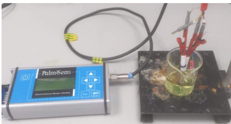
Figure 2.17: The equipment setup for the CV measurements using a PalmSens potentiostat and a three electrode circuit.
