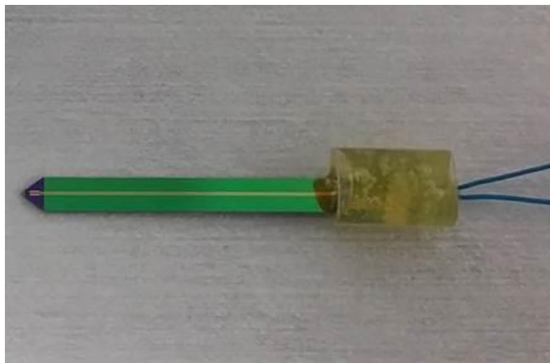
Figure 2.12: A packaged probe showing the plastic tubing filled with hardened 2-part epoxy covering the electrical connects.
