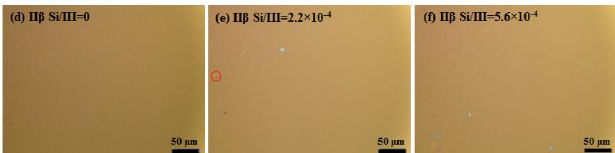
Figure 6.7: Nomarski optical microscope images of selected AlGaIn samples from Series II \alpha and II \beta , respectively. Micro-scale defects are indicated by red circles.
