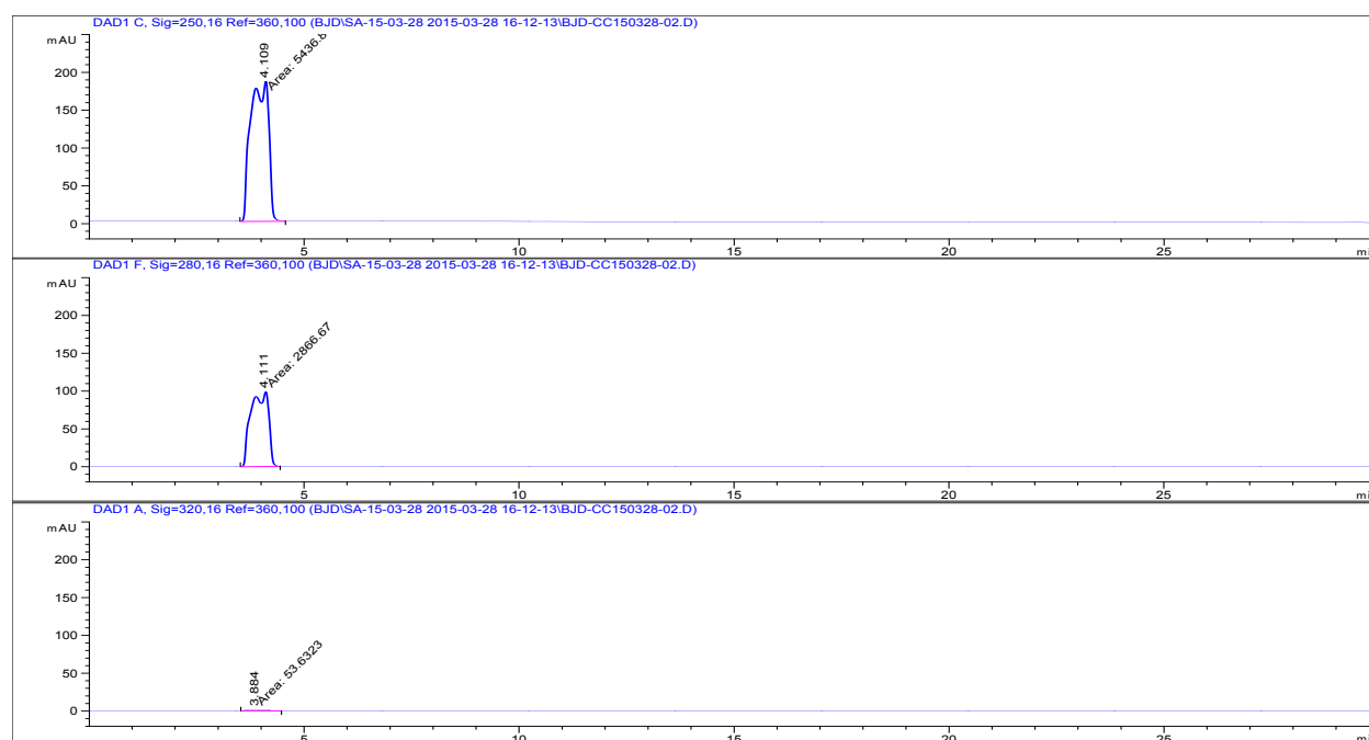
Figure 45. HPLC analysis of isonicotinic acid measured at 250 nm (top), 280 nm (middle) and 320 nm (bottom) (INC).
