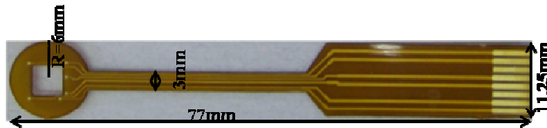
Figure 3.2. Flexible substrate with window opening for sensor access.
