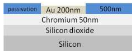
Figure 2.11. Schematic of deposited stack layer of the microelectronics sensor.
