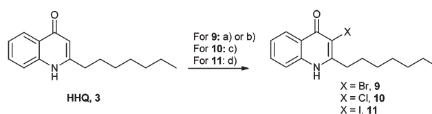
Scheme 3 Halogenation of HHQ. Conditions: (a) NBS, MeOH, 37% (b) Br 2 , AcOH, 47% (c) DCIC, H 2 O, 46% (d) NIS, AcOH, 48%.
